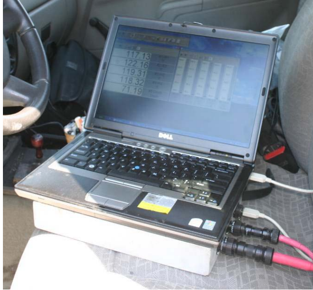
Figure 3-6 Laptop based data collection system shaded in field vehicle.
