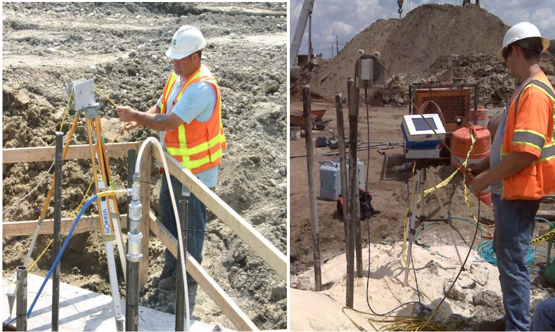
Figure 3-5 Tripod-mounted depth wheel (left) tube-mounted depth wheel (right).
