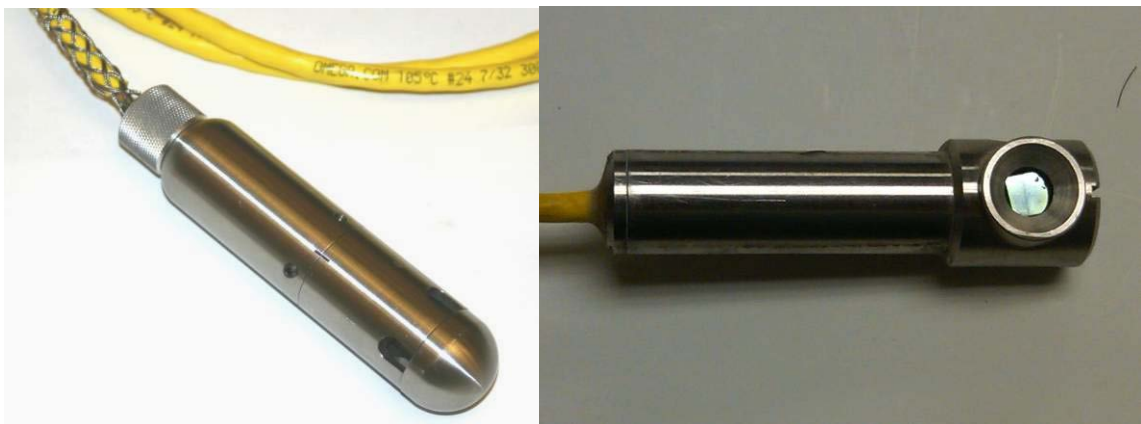
Figure 3-4 Thermal probe (left) encased infrared sensor (right).
