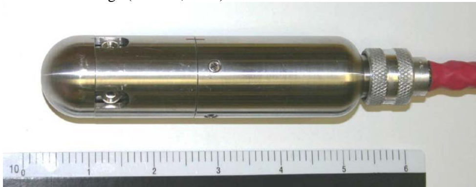
Figure 2-4 TIP probe equipped with four infrared thermocouples.
