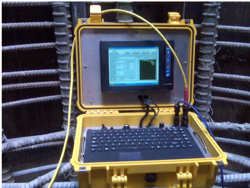
Figure 3-6 Ruggedized data collection system with waterproof keyboard and screen.
