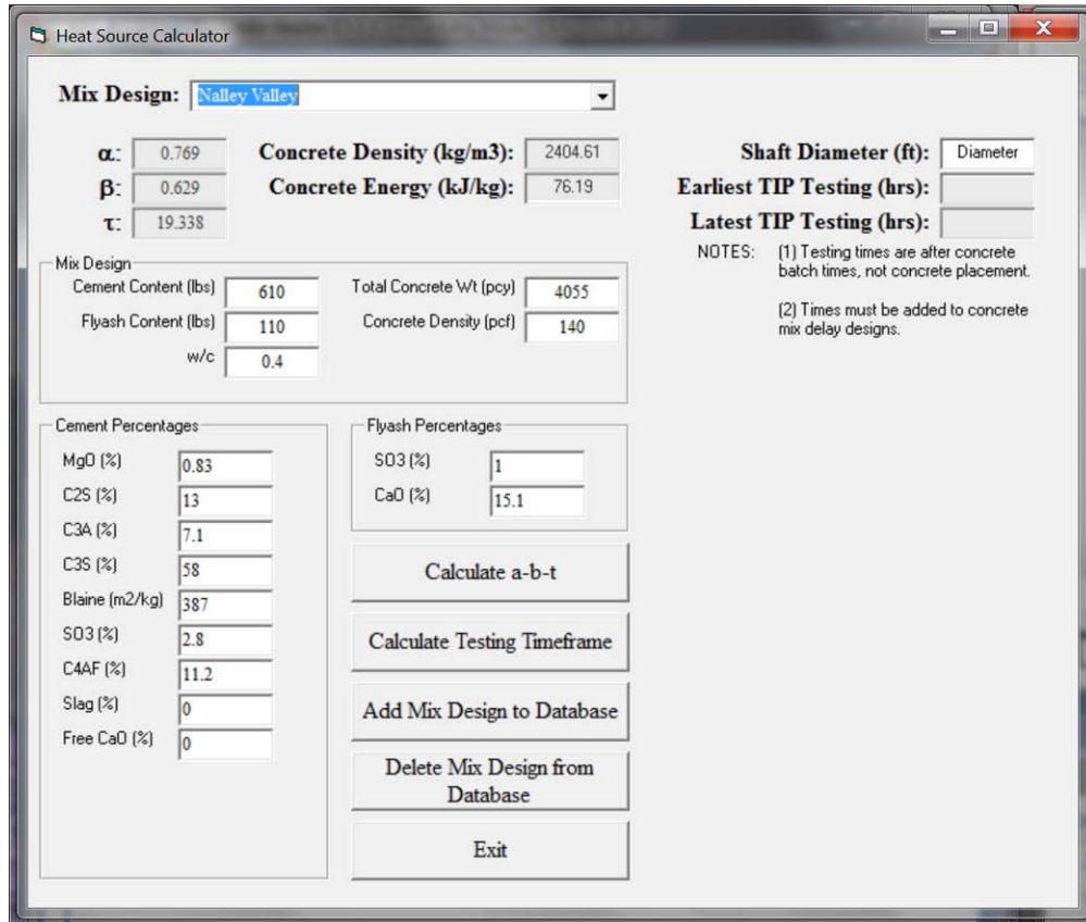
Figure 3-1. Heat Source Calculator used to define the testing time window.
