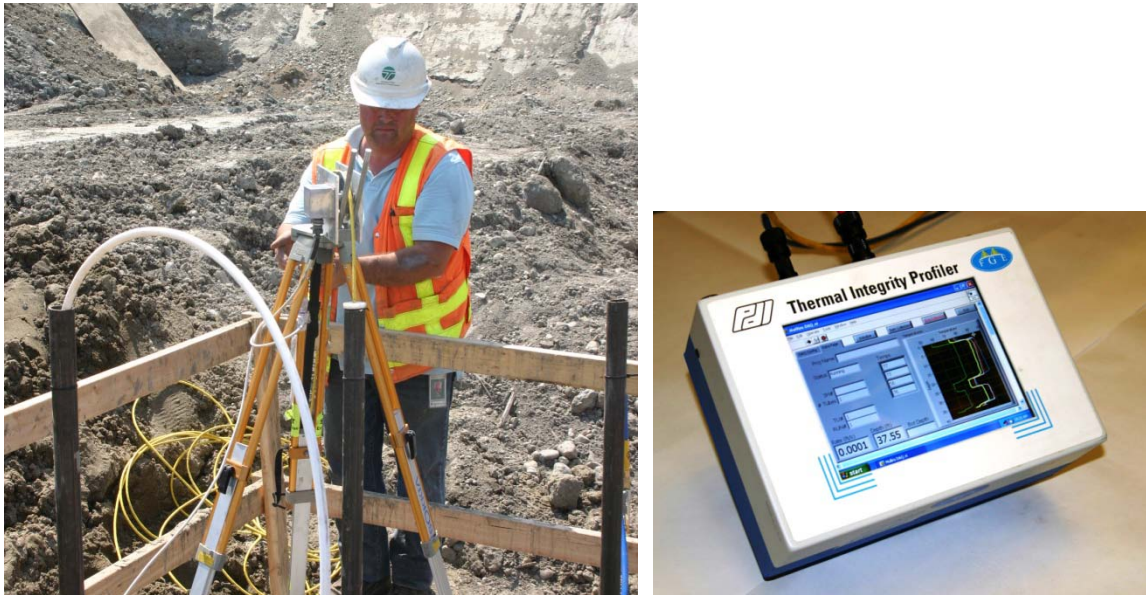
Figure 2-5 Thermal integrity profiling (left) data collection computer (right).
