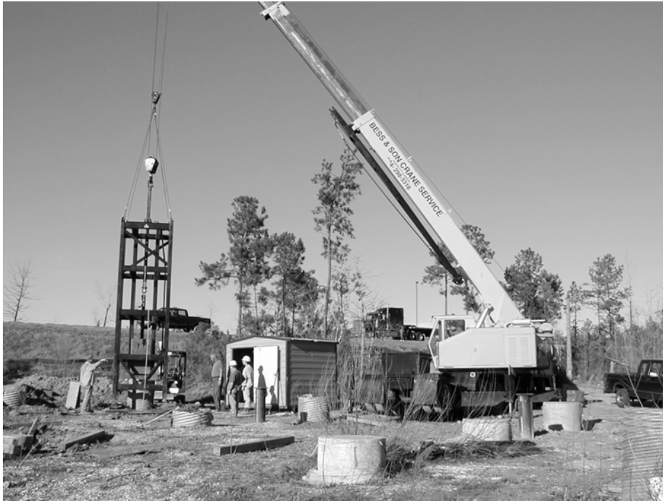
Figure 7: Tests on a Corrugated Drilled Shaft at the Auburn Site.
