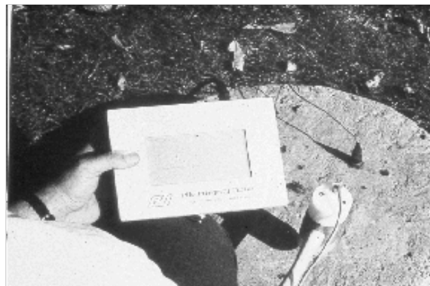
Figure 3. Pile Integrity Tester (PIT) system with hammer and accelerometer (upper right).
