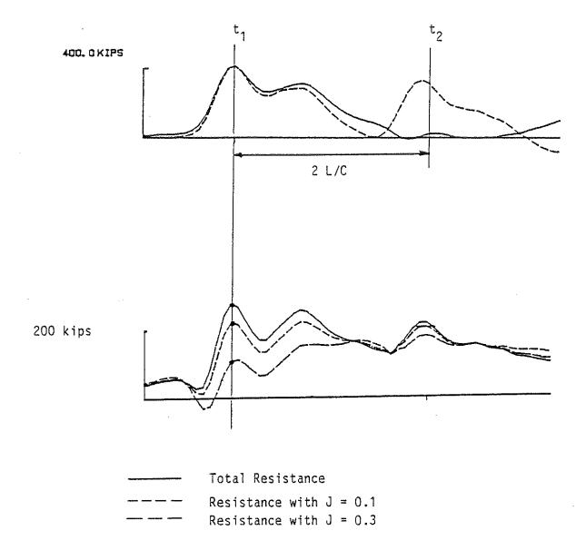
From Resistance - time Curve: RTL = 275 kips RS1, with J = 0.3, = 108 kips
