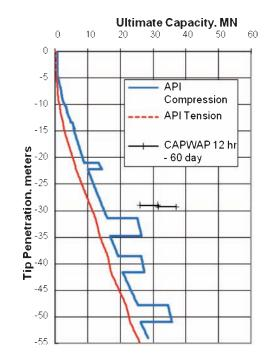
Figure 6. Site D Pile capacity from API and DMS results.
