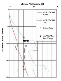
Figure 5. Pile capacity from API prediction, DMS results and pile pull out tests.
