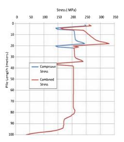
Figure 1. Site A Pile Stress Profile.
