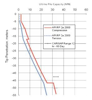
Figure 2. Site A static vs DMS capacities.
