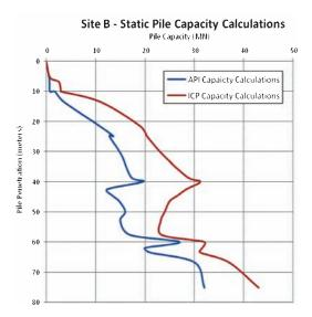
Figure 3. API & ICP static pile capacity calculations.
