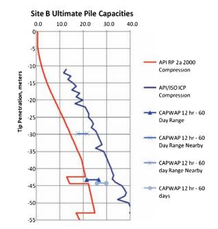
Figure 4. API, ICP and DMS pile capacities.
