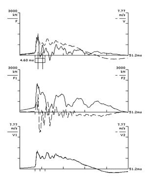
Figure 1a. Data with a loose strain transducer.
