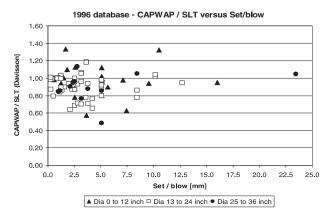
Figure 2. Ratio of CAPWAP to SLT prediction versus permanent set per blow.
