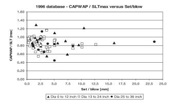
Figure 3. Ratio of CAPWAP to max applied load in SLT vs. set per blow.
