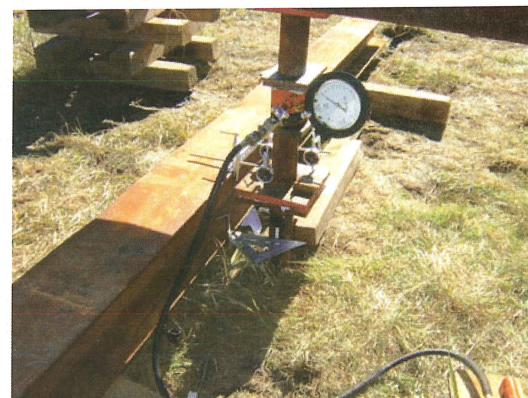
[FIG. 8] Static Load Test setup
