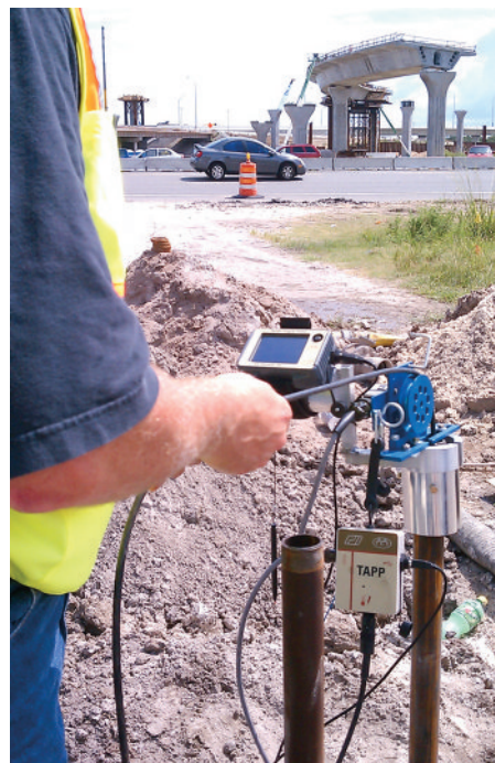
Figure 3. Thermal probe system used to perform thermal integrity profiles (probe shown below)
