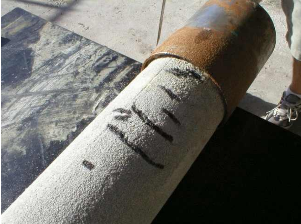
Figure 4-25. Surface Cracking in Upper Portion of Shaft Specimen
