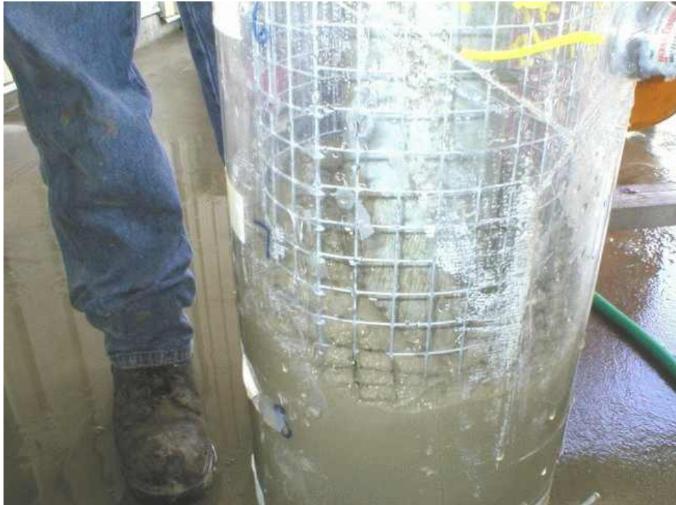
Figure 3-19. Head Differential Using 1/2" Cage, Dry Hole Construction
