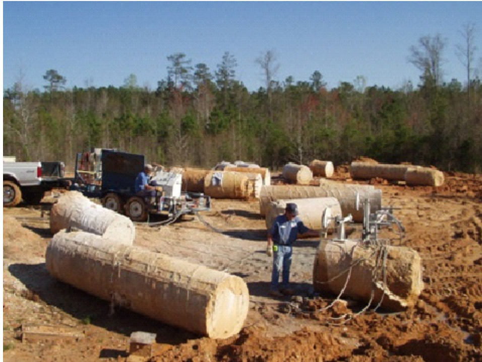
Figure 6-67. Saw Cutting of Test Shafts
