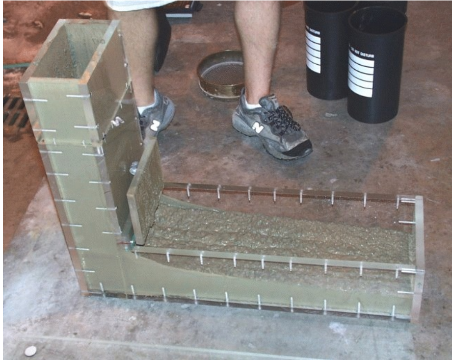
Figure 6-19. Material Flows Through Lower Gate and Drop Height Is Recorded
