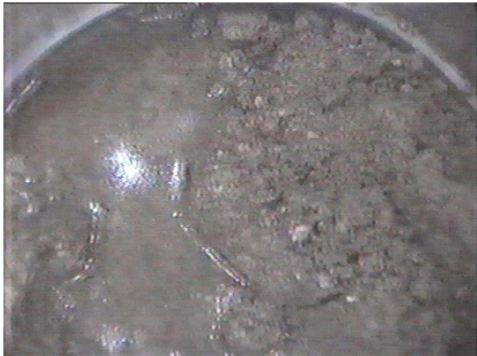
Figure 6-20. TS-1: Borehole Cleanliness as Observed with the Borescope
