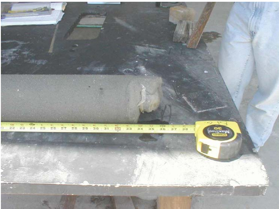
Figure 4-22. Uneven Toe Formation on Shaft S8
