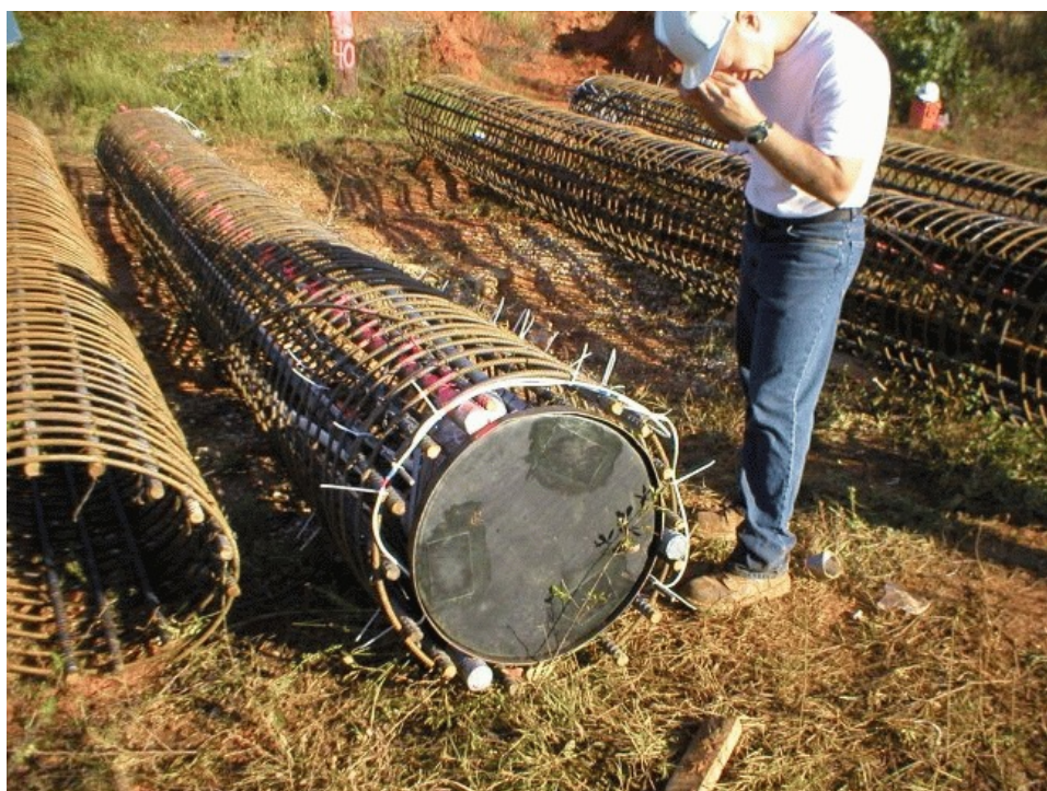
Figure 6-4. Post Grout Cell as Installed in Auburn Test Shaft
