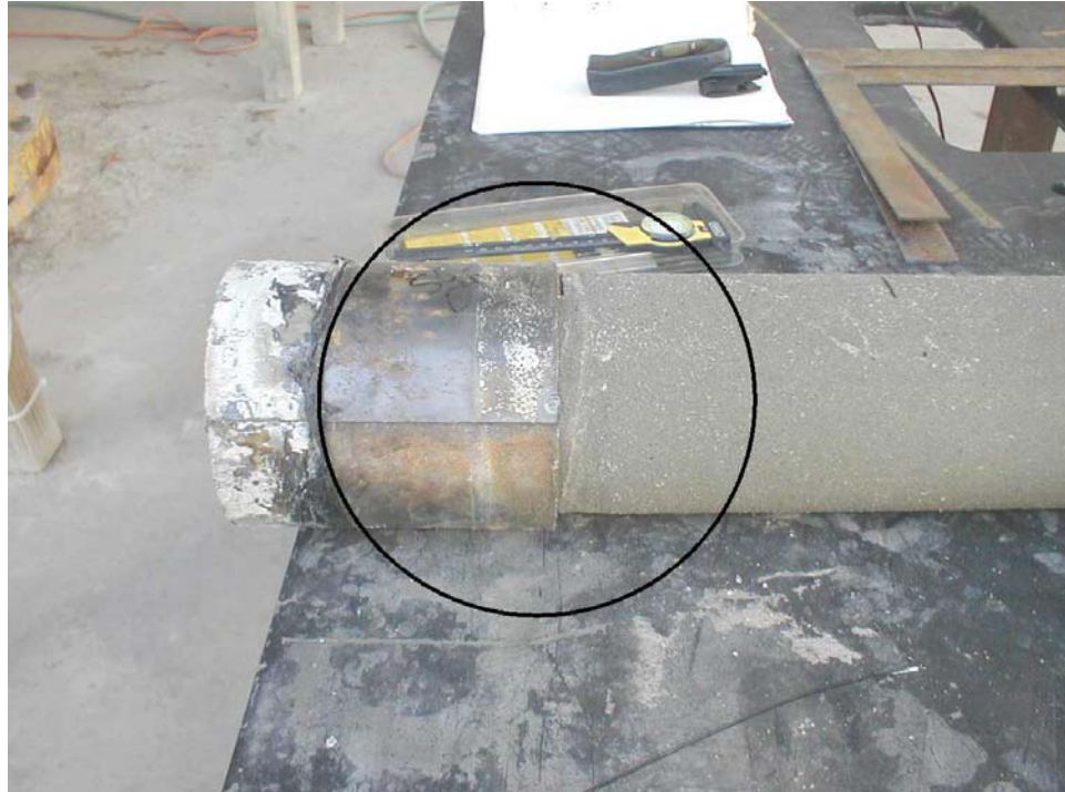
Figure 4-19. Slight Neck below Casing on Shaft S5
