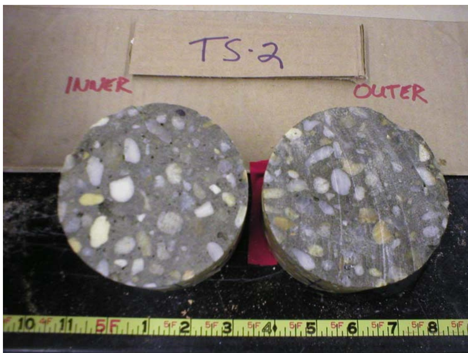
Figure 6-71. Core Sample from Shaft TS-2
