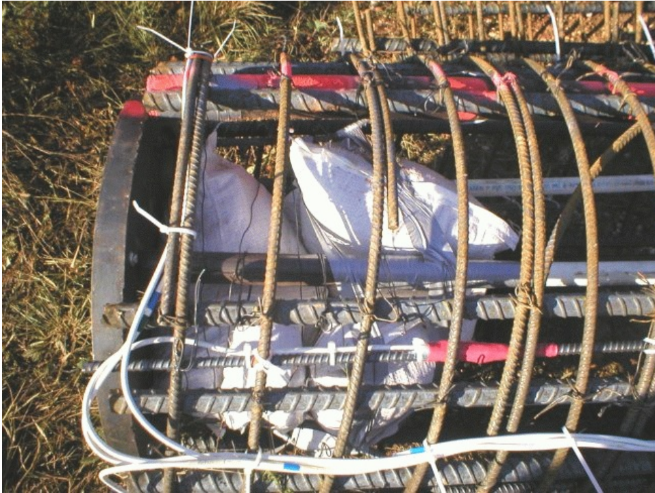
Figure 6-5. Toe Anomaly Created by Installing Sand Bags Inside the Cage
