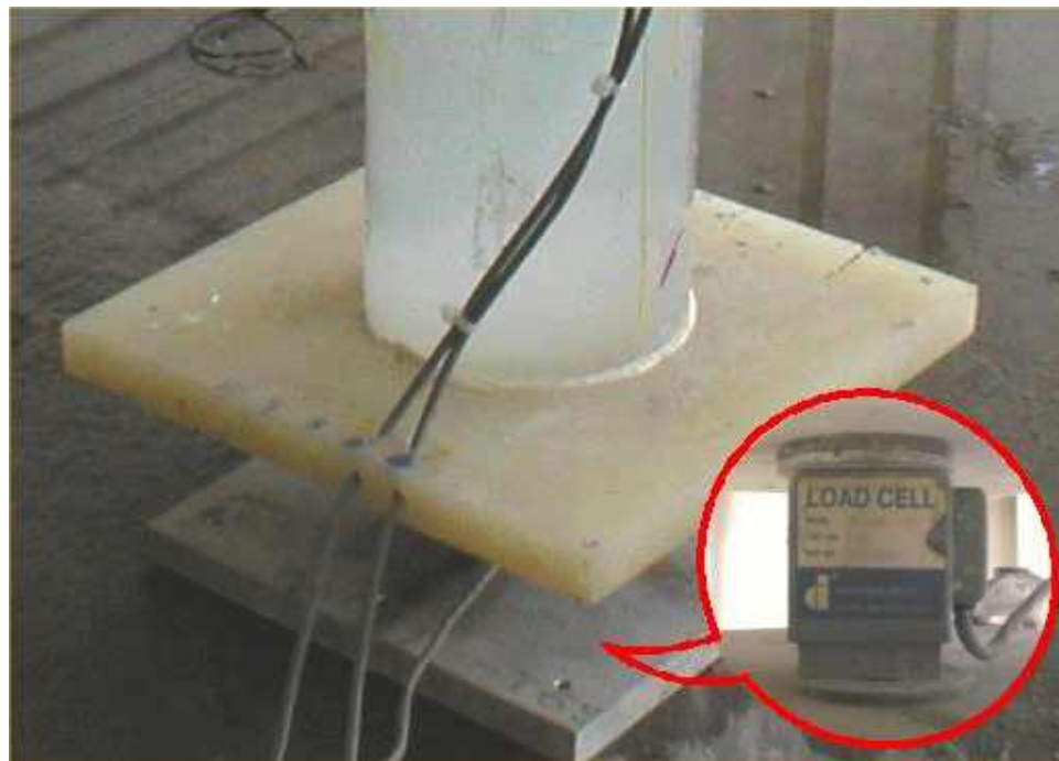
Figure 3-4. Load Cell (inset) is Mounted Between the Base Plates
