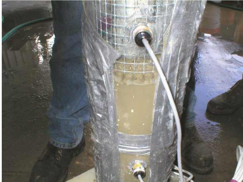
Figure 3-3. Lateral Pressure Transducers Mounted to LPC Side Wall
