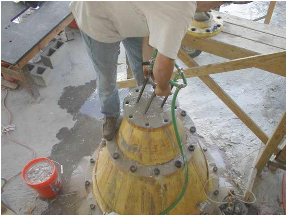
Figure 4-2. Alluviation of the FCV Using the Water Jet Tool
