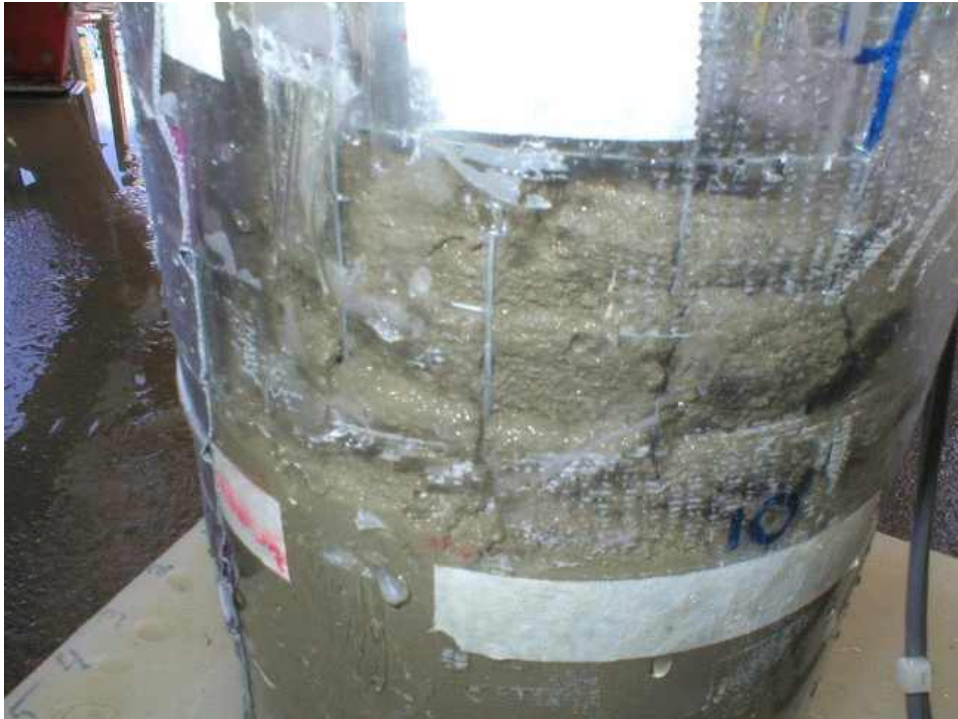
Figure 3-21. Head Differential Using 1" Cage, Dry Hole Construction
