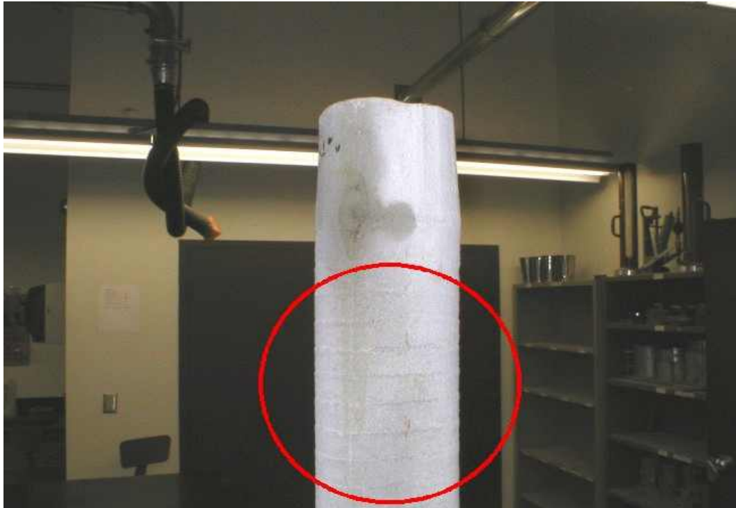
Figure 4-27. Surface markings due to casing wobble during extraction on Shaft S32
