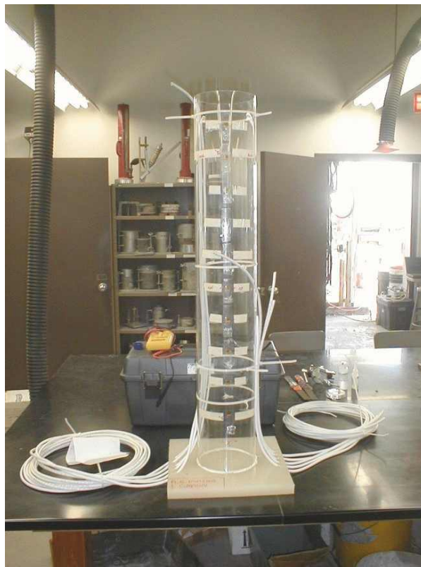
Figure 3-2. Resistive Strain Gages Mounted
