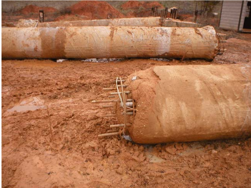
Figure 6-43. TS-4 Exhumed Shaft Tip
