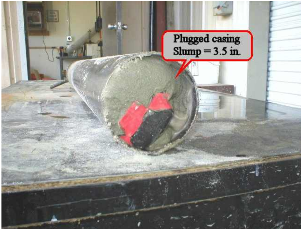
Figure 4-29. Entire Shaft Lodged in Casing Due to Excessive Slump Loss on Shaft S47
