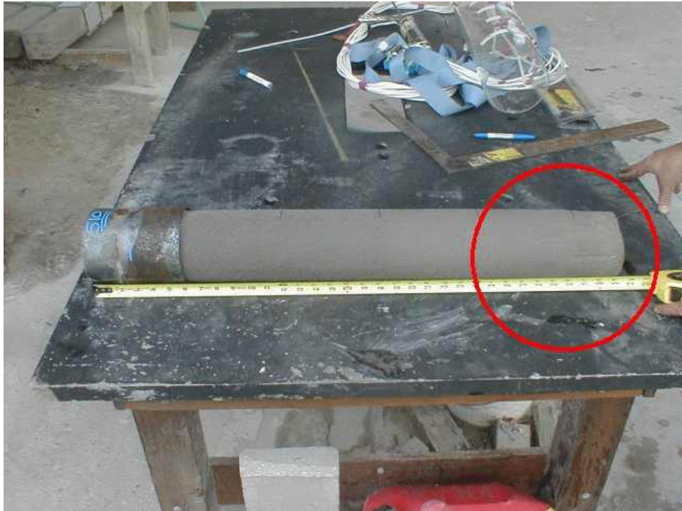
Figure 4-23. Reduced cross section at toe Shaft S10
