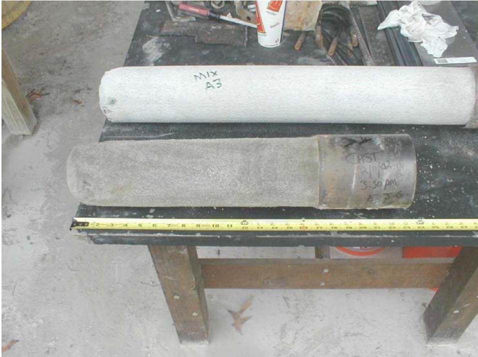
Figure 4-17. Shaft S1 Removed from the Frustum - Undersized
