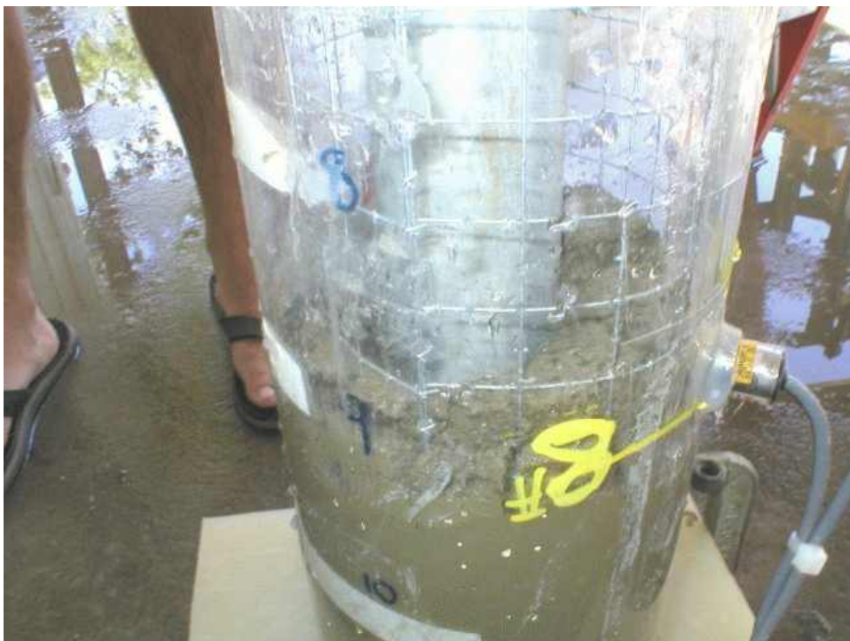
Figure 3-22. Alternate View of Head Differential Using 1" Cage, Dry Hole
