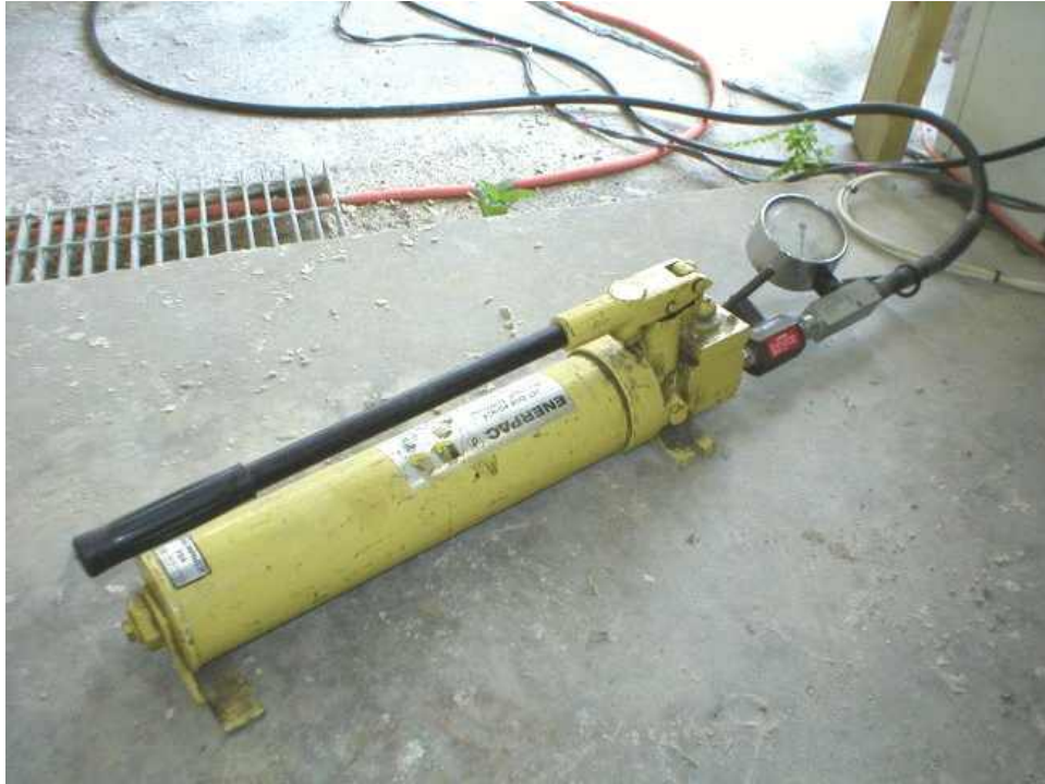
Figure 4-15. Manual Pump Used to Control Hydraulic Jack
