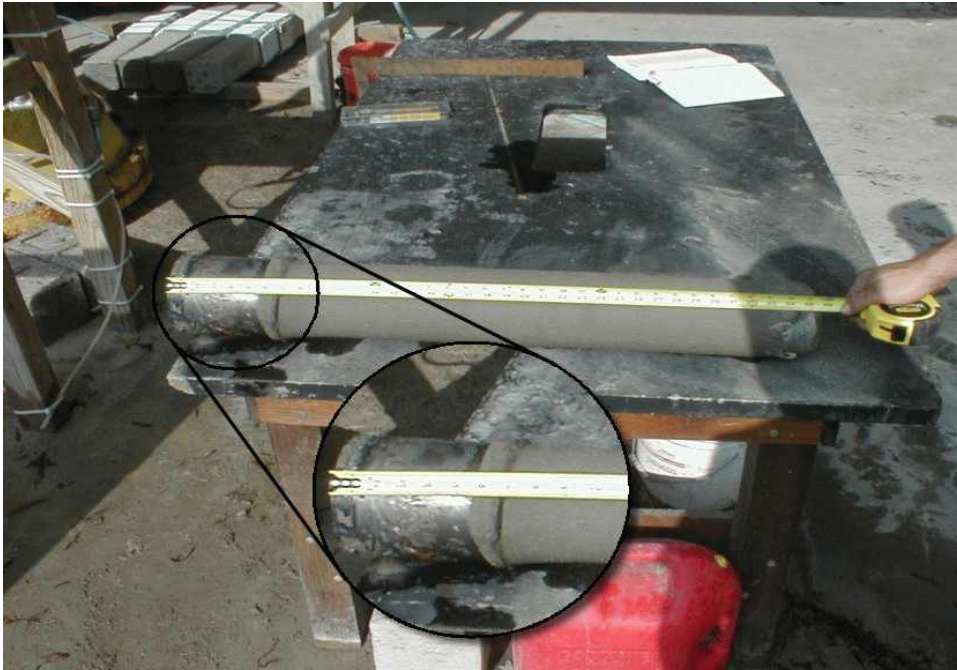
Figure 4-21. Shaft S7 Showing Bulge Just below Permanent Casing
