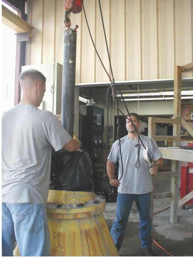
Figure 4-9. Casing Extraction Using the Overhead Lift
