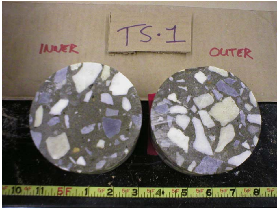
Figure 6-69. Core Sample from Shaft TS-1 Showing Material from Inner & Outer Cage
