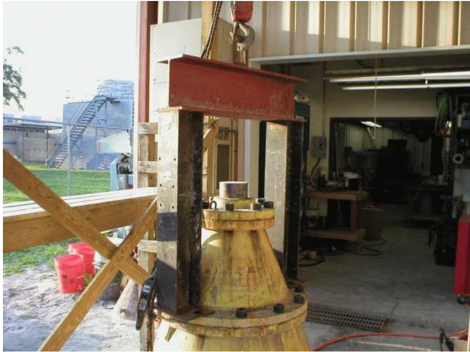
Figure 4-11. Reaction Frame Used for FCV Static Load Testing
