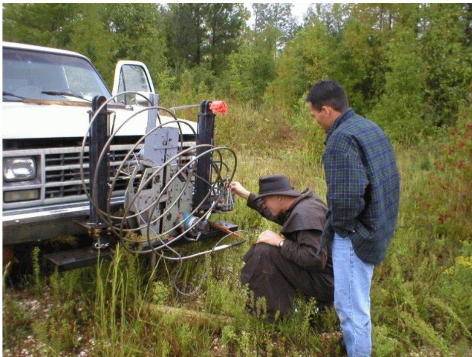
Figure 6-9. Subsurface Exploration Using the USF Mini-CPT Rig
