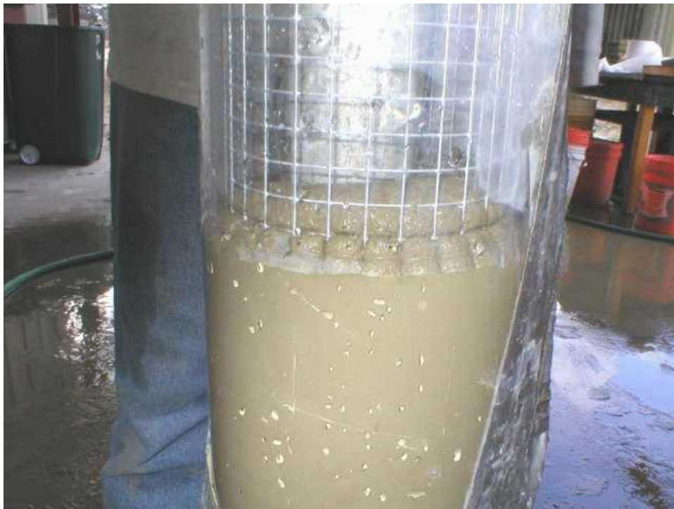
Figure 3-30. One Inch Head Differential in an Early LPC Pour
