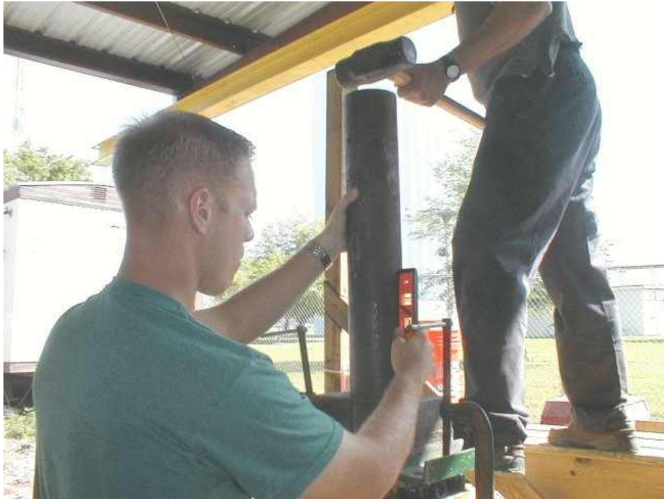
Figure 4-3. Casing Driven into Specified Depth
