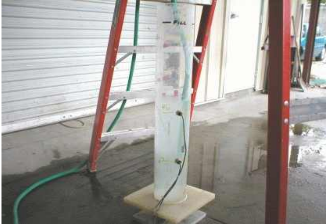
Figure 3-5. Water Calibration of the Lateral Pressure Cell Prior to Mortar Testing
