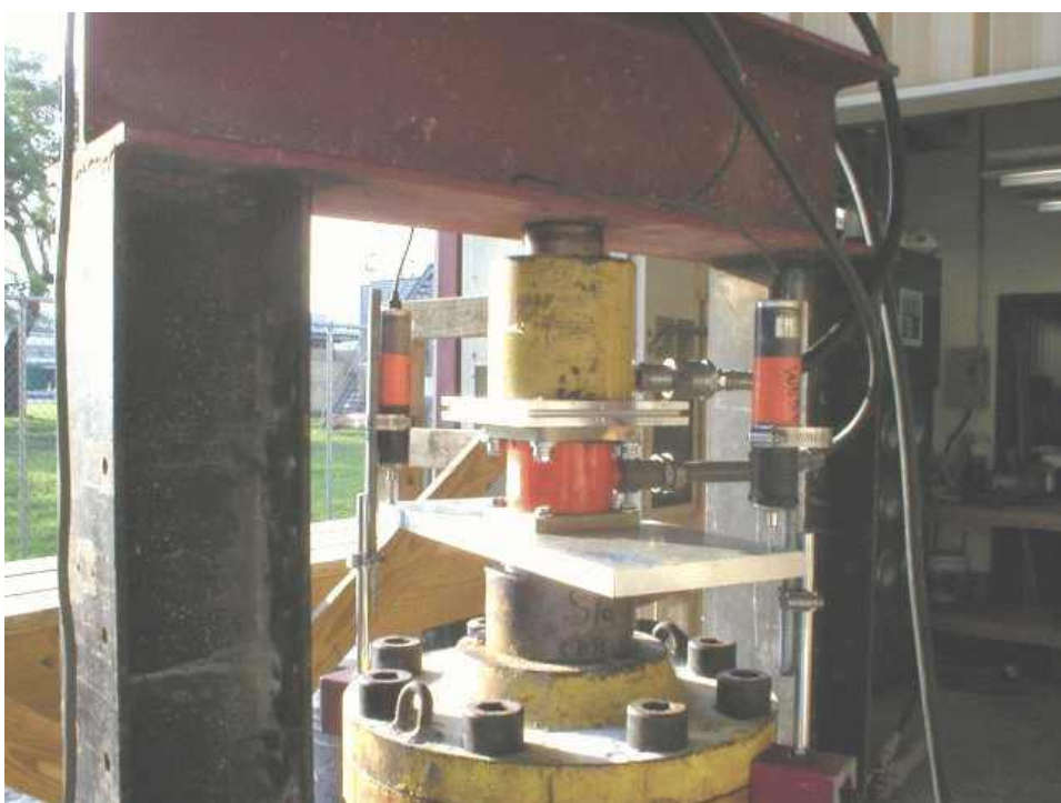
Figure 4-14. Hydraulic Jack and LVDTs Installed on Shaft
