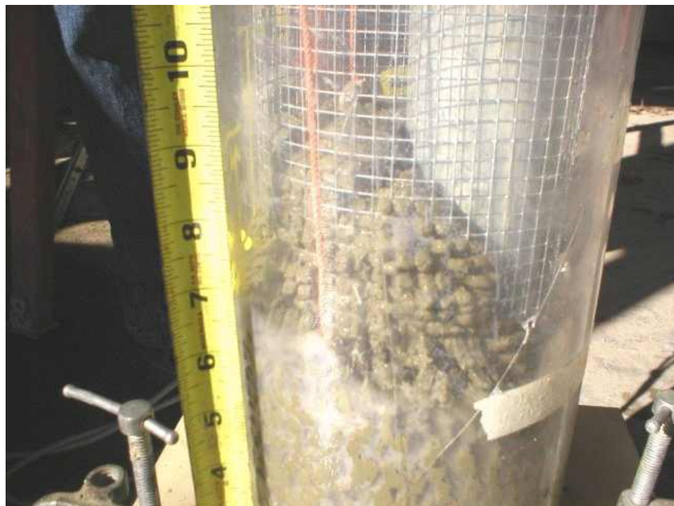
Figure 3-16. Head Differential Using 1/4" Spacing, Dry Hole Construction
