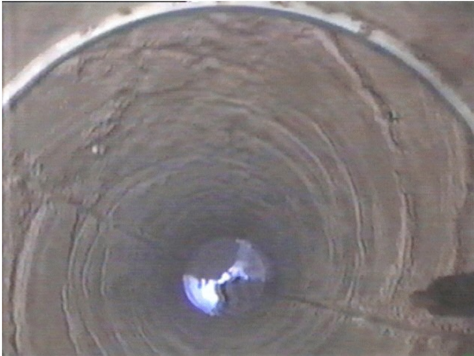
Figure 6-21. TS-1: Sidewall of Borehole Viewed with Borescope
