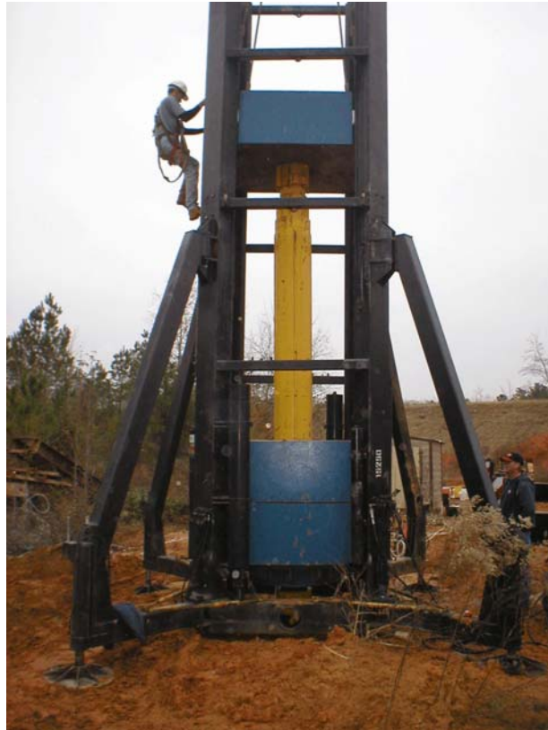
Figure 6-63. 4MN Statnamic Load Test Setup
