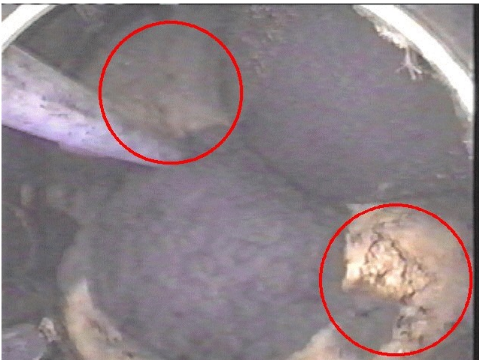
Figure 6-30. TS-3: #57 Stone, Low Slump, Showing Segregation and Bleeding
