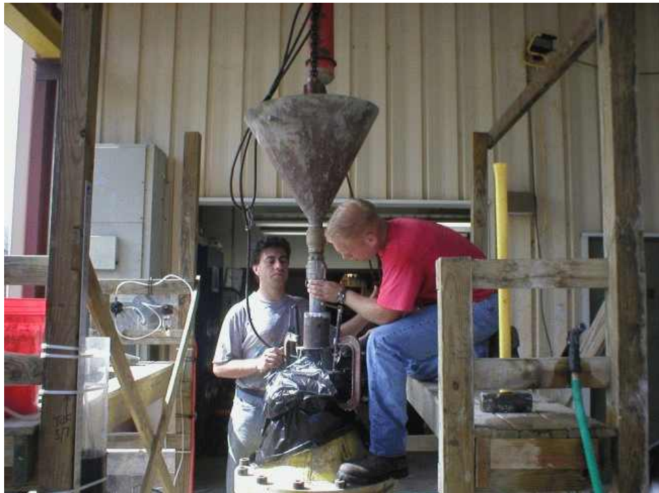
Figure 4-8. Connecting Tremie Pipe to Hopper in Preparation for Pour
