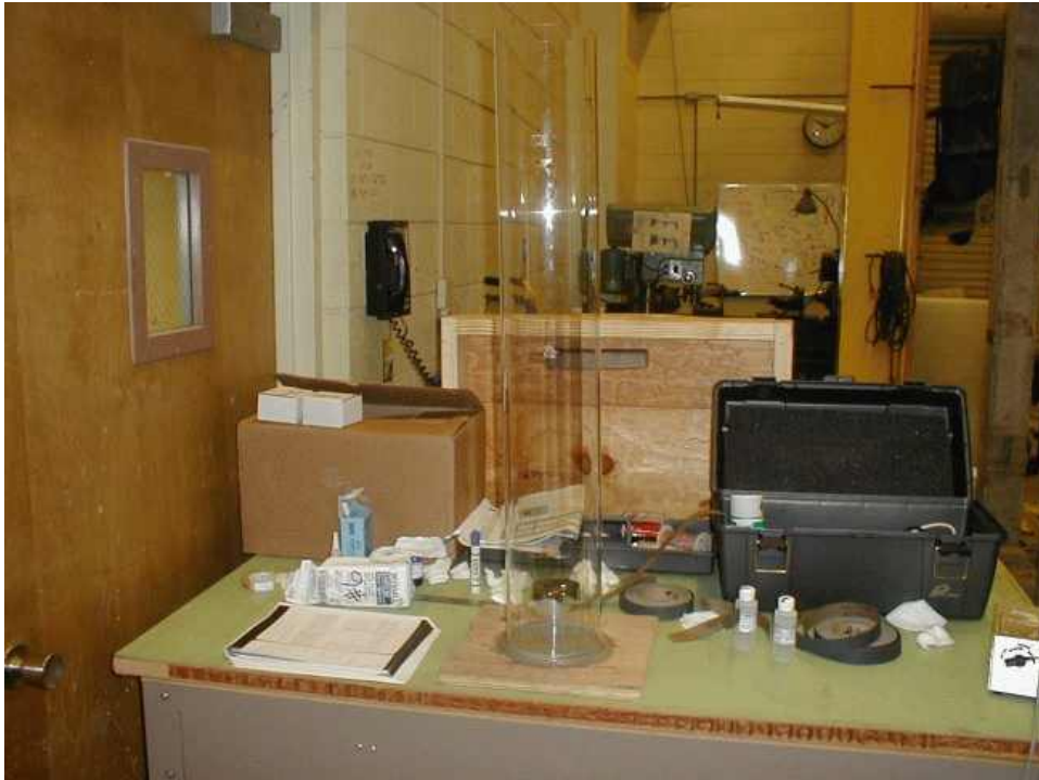
Figure 3-1. Lucite Tube Used to Construct the Lateral Pressure Cell
