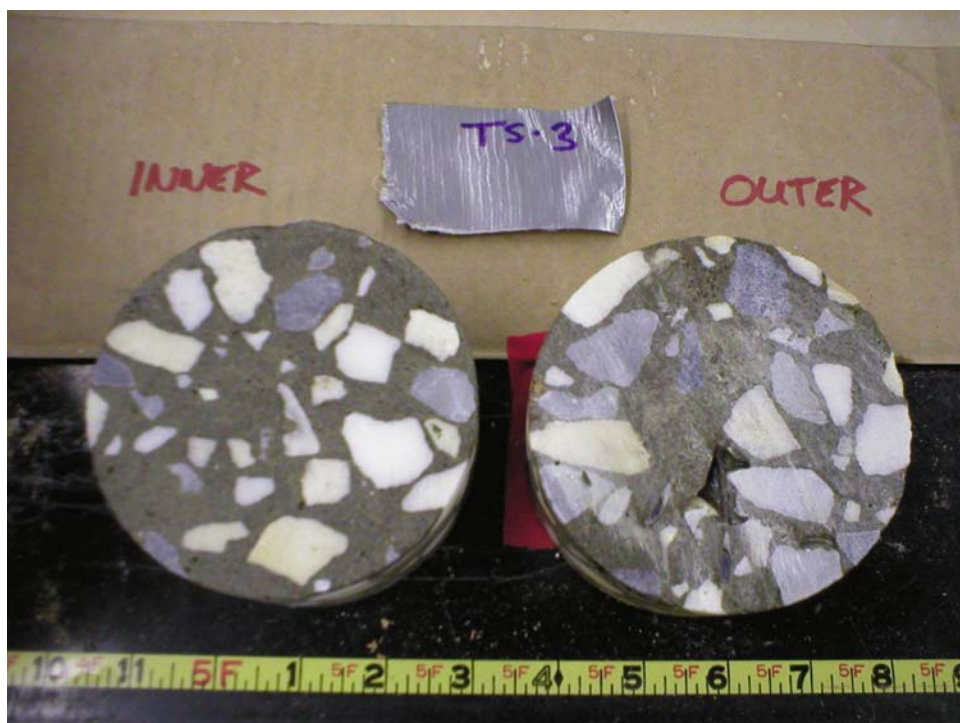
Figure 6-72. Core Sample from Shaft TS-3
