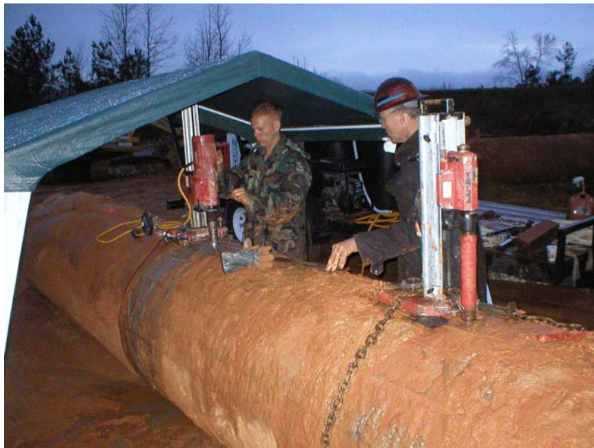
Figure 6-66. Coring of Test Shafts for Permeability Testing
