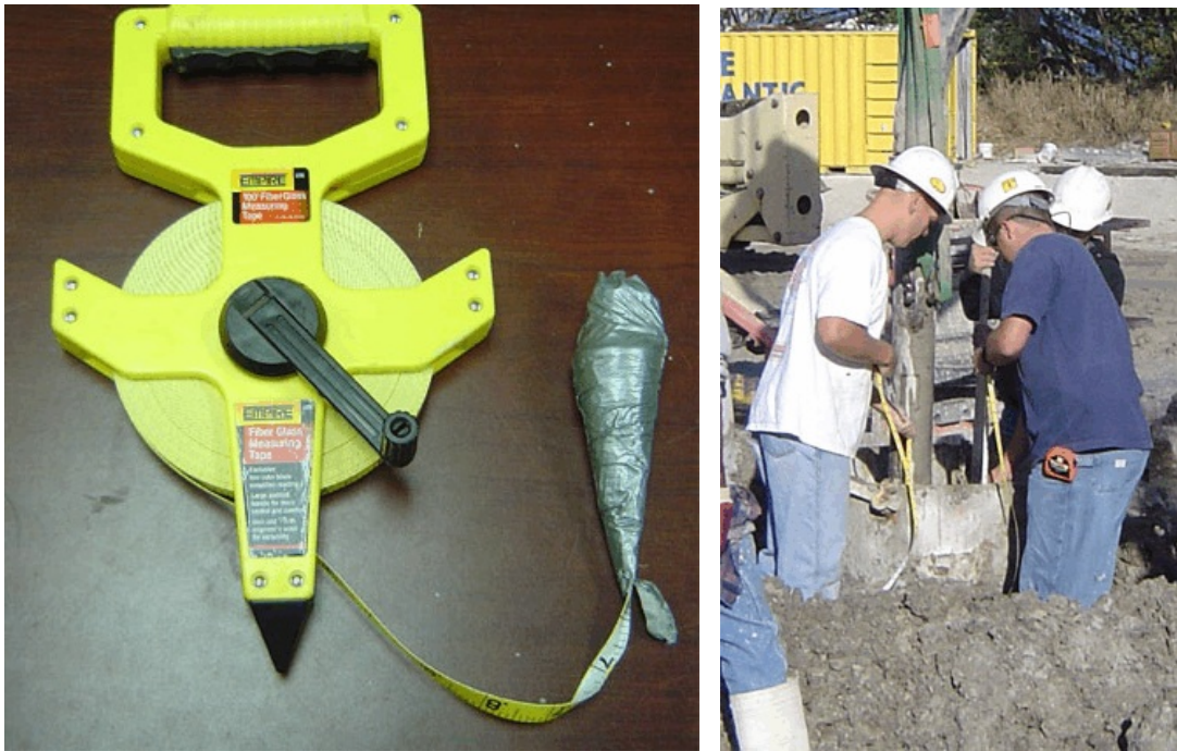
Figure 7-1. Weighted Tape (left) used in Taking Head Differential Measurements (right)
