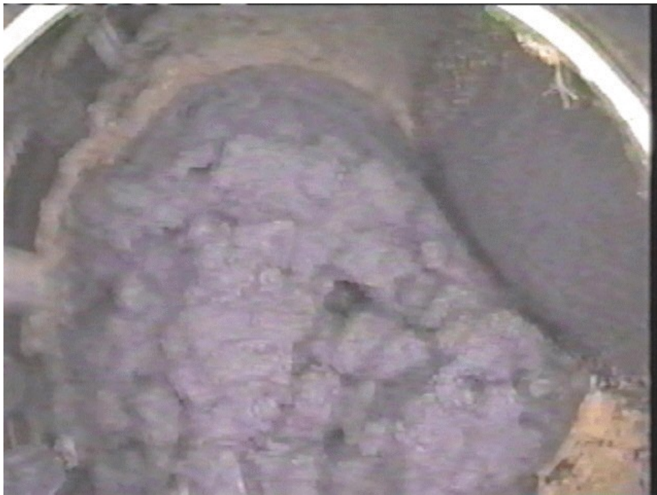
Figure 6-32. TS-3: Low Slump Mix Also Exhibits High Degree of Clumping
