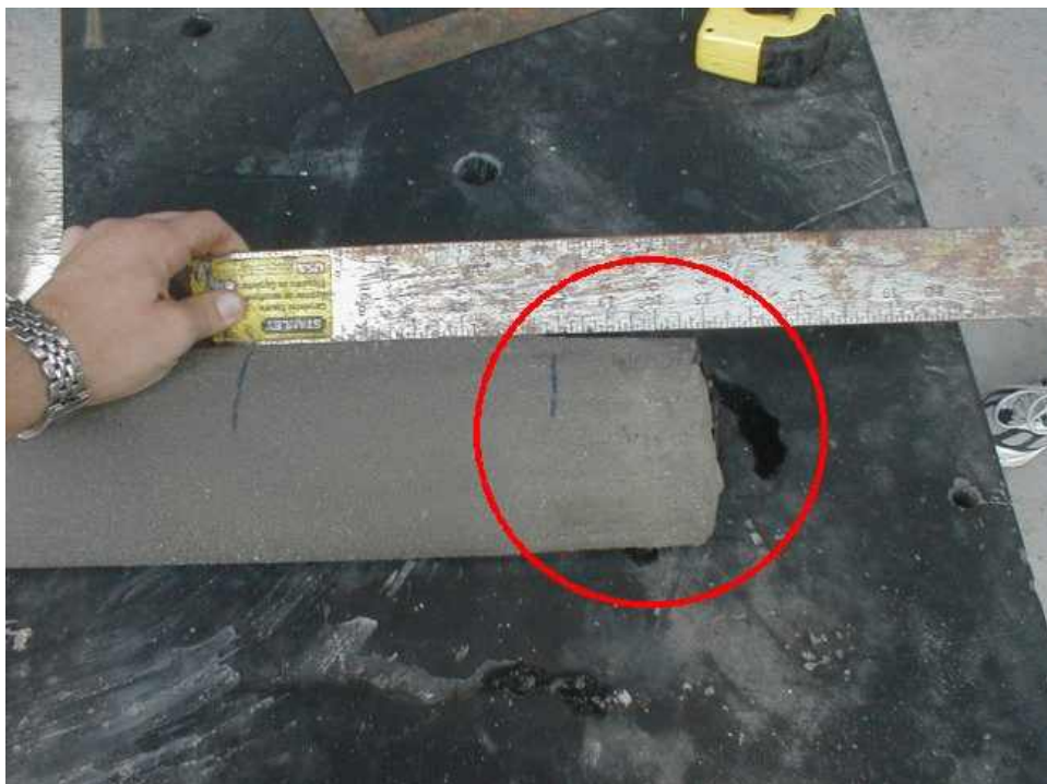
Figure 4-24. Reduced toe cross-section due to poor excavation on Shaft S40
