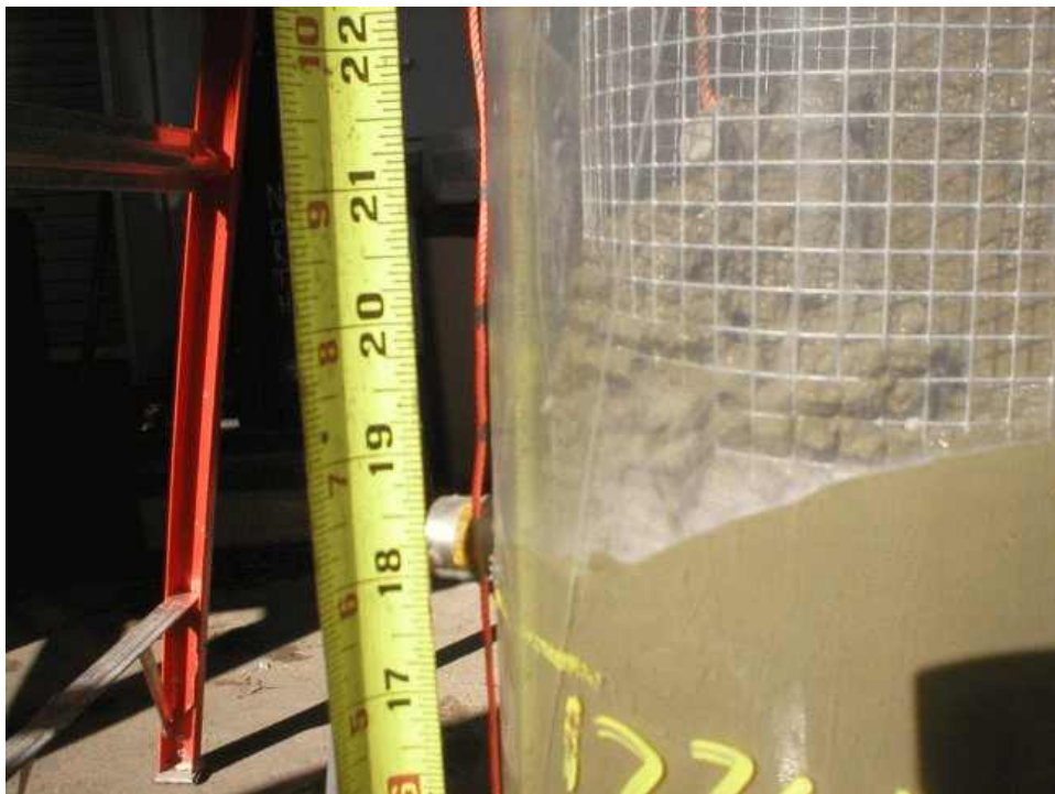
Figure 3-18. Flow past Lateral Pressure Transducer with Obvious Head Differential
