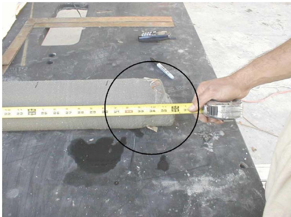
Figure 4-20. Toe Anomaly on Shaft S5
