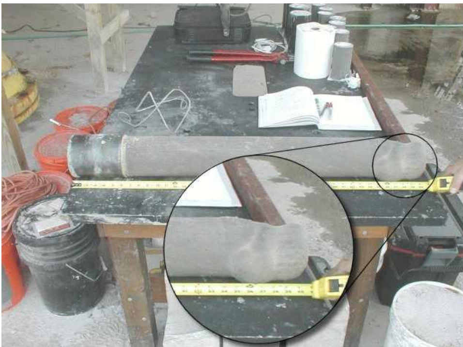
Figure 4-18. Toe Bulb on Shaft S2 due to Over-excavation
