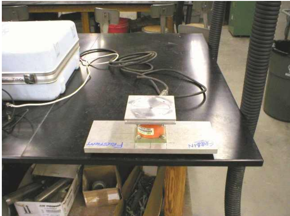
Figure 4-12. Load Cell and Bearing Plates used for FCV Static Load Testing
