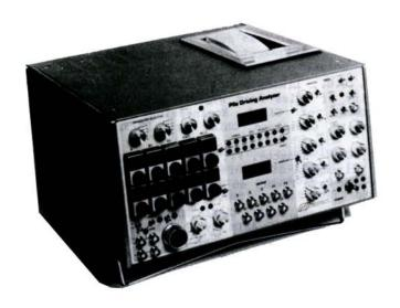
FIGURE 1: PILE DRIVING ANALYZER
