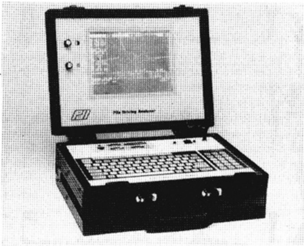
Figure 2: The Pile Driving Analyzer® (PDA)
