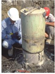
Figure 2: Stain gauges and accelerometers attached at the shaft top
