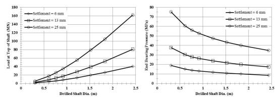
Figure 1. Drilled shaft (a) load and (b) end bearing pressure as a function of diameter and elastic settlement
