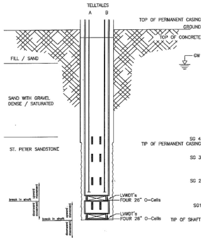
Figure 2. Test Shaft Arrangement (Loadtest, 2007)
