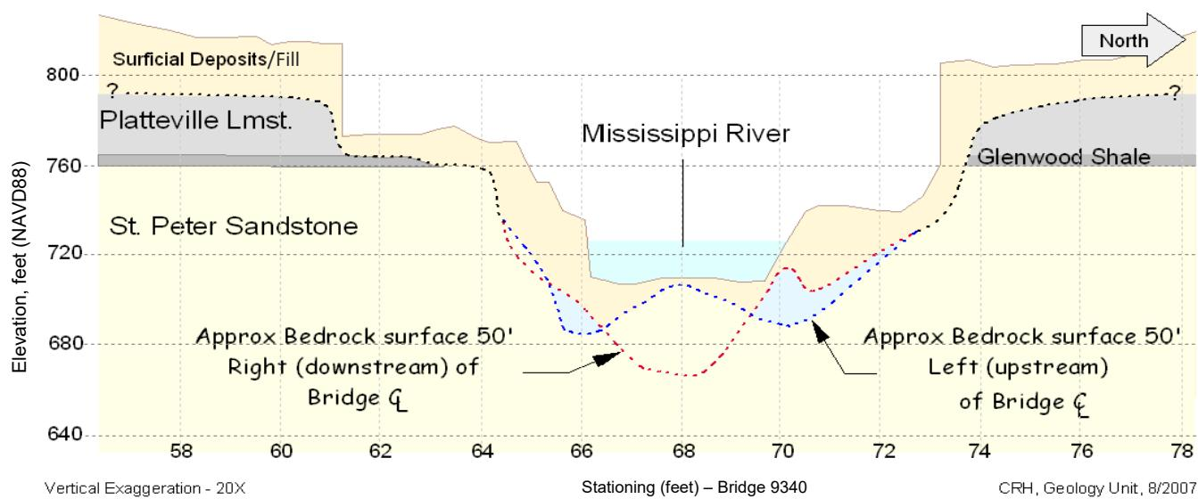
Figure 1. Generalized Subsurface Conditions (MnDOT, 2007)
