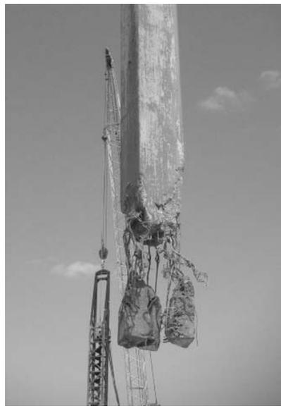
Figure 8. Extracted concrete pile showing the pile damage.
