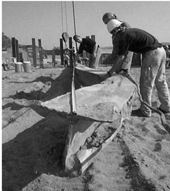
Figure 11. Extracted pile with near-toe damage.
