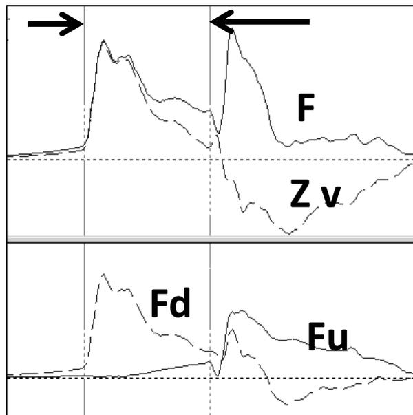
Figure 9. H pile driven to refusal at penetration of 59 ft (18 m).
