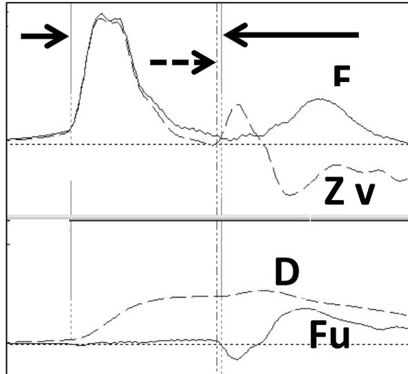
Figure 7. Concrete pile at blow number 1420, 300 blows after first damage detection.
