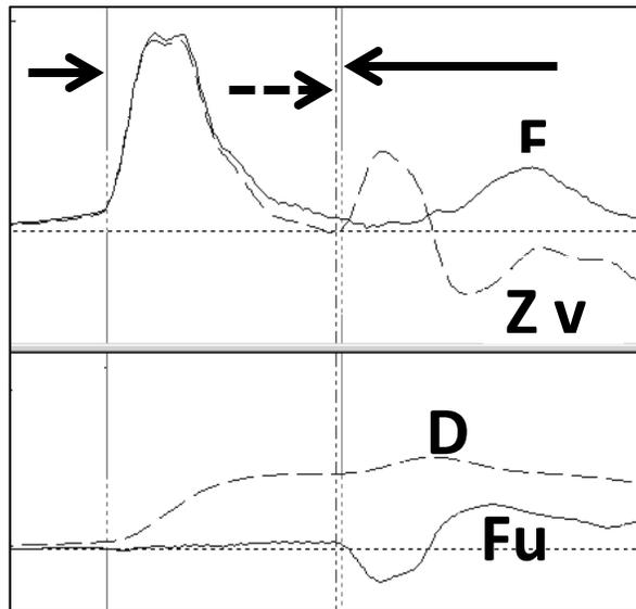
Figure 6. Prestressed concrete pile, a few blows after first damage detection.
