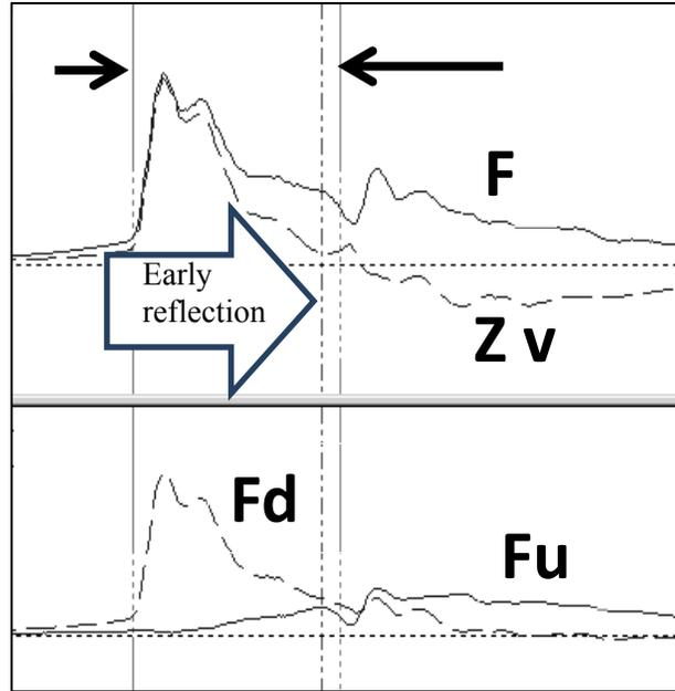
Figure 10. Pile driven to 78 ft (23.8 m) demonstrates near-toe damage.
