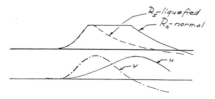
Figure 2: Static resistance, Pile Velocity and Displacement for Liquefying Soil
