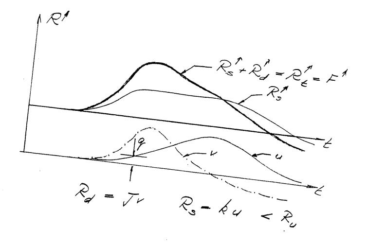
Figure 1: The Basic CAPWAPC Matching Process
