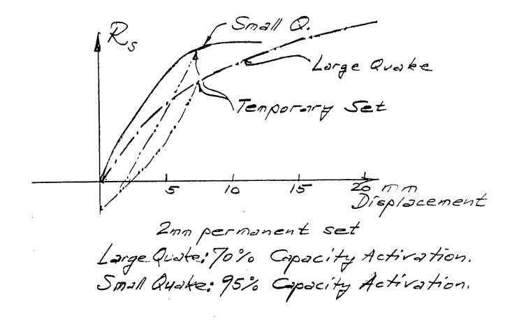
Figure 3: Load-Set Curves for Partial Activation
