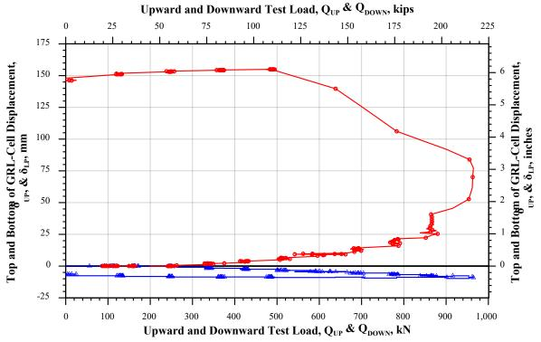
Figure 4. TDDP-1 jack assembly load-displacement plot.
