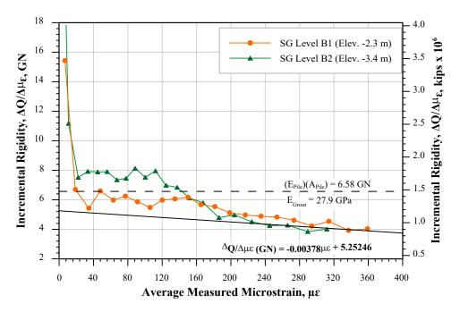
Figure 6. Incremental Rigidity versus Strain for interpretable SG Levels in TACIP-1.
