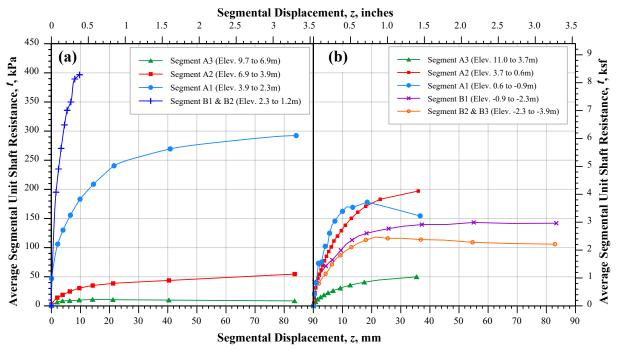
Figure 8. Load transfer results, displaying t-z curves for (a) TDDP-1, and (b) TACIP-1.
