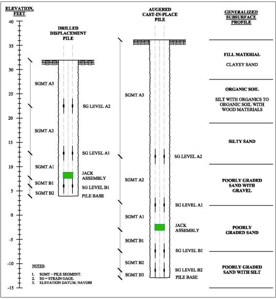
Figure 2. Pile installations elevation views.
