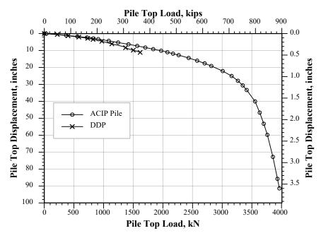
Figure 10. ETL Curves Comparison.
