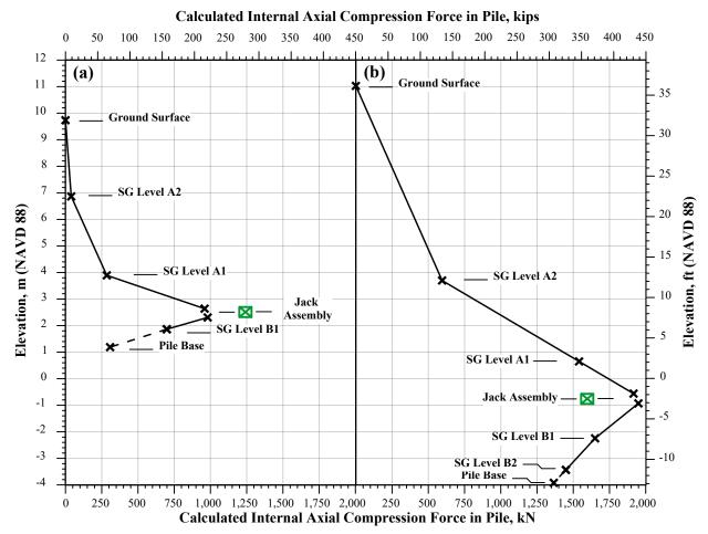
Figure 7. Internal force profiles at the maximum achieved bi-directional test load for (a) TDDP-1, and (b) TACIP-1 using the IR method.
