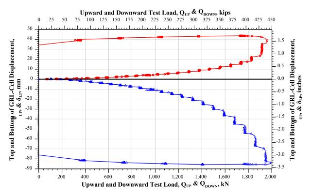
Figure 5. TACIP-1 jack assembly load-displacement plot.
