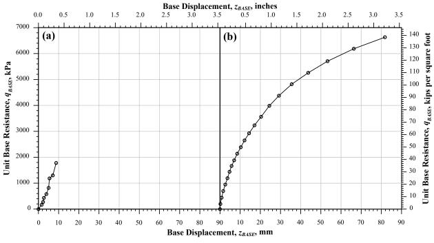
Figure 9. Load transfer results displaying *q<sub>BASE</sub>-z<sub>BASE</sub>* curves for (a) TDDP-1, and (b) TACIP-1.
