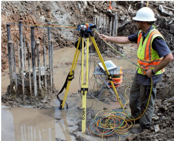
Figure 15. Typical field set-up of CSL test.
