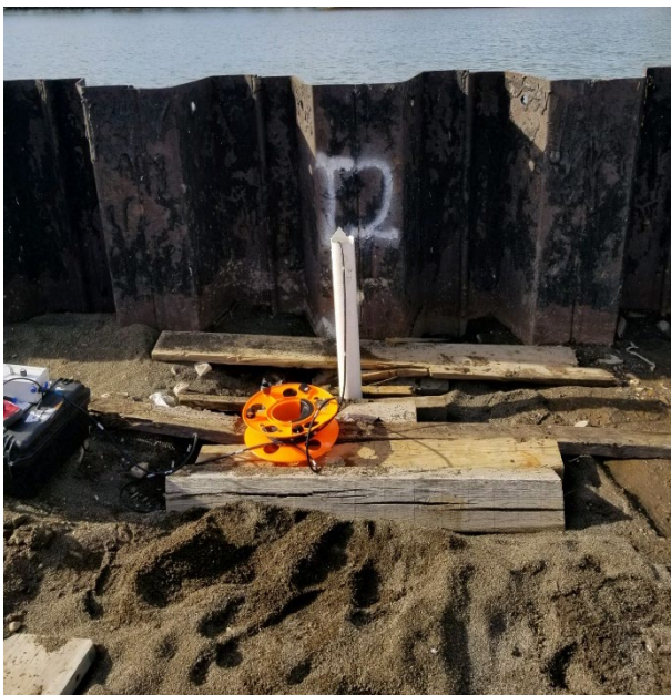
Figure 43 LITE probe in PVC borehole.
