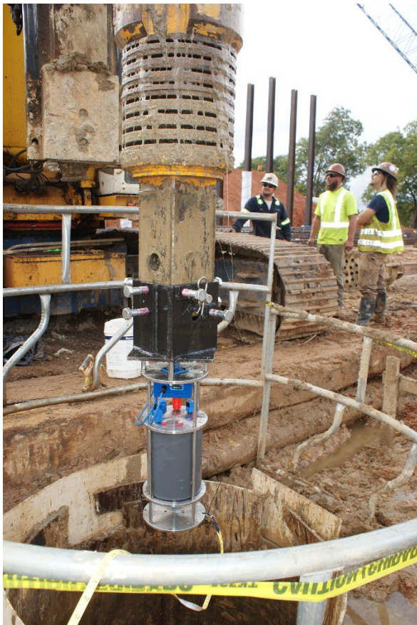
Figure 30. SHAPE moving over shaft excavation.
