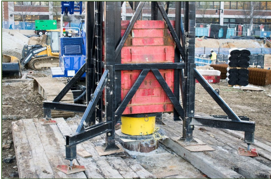
Figure 5. APPLE system configured with 44 ton drop weight and load cell positioned atop drilled shaft.
