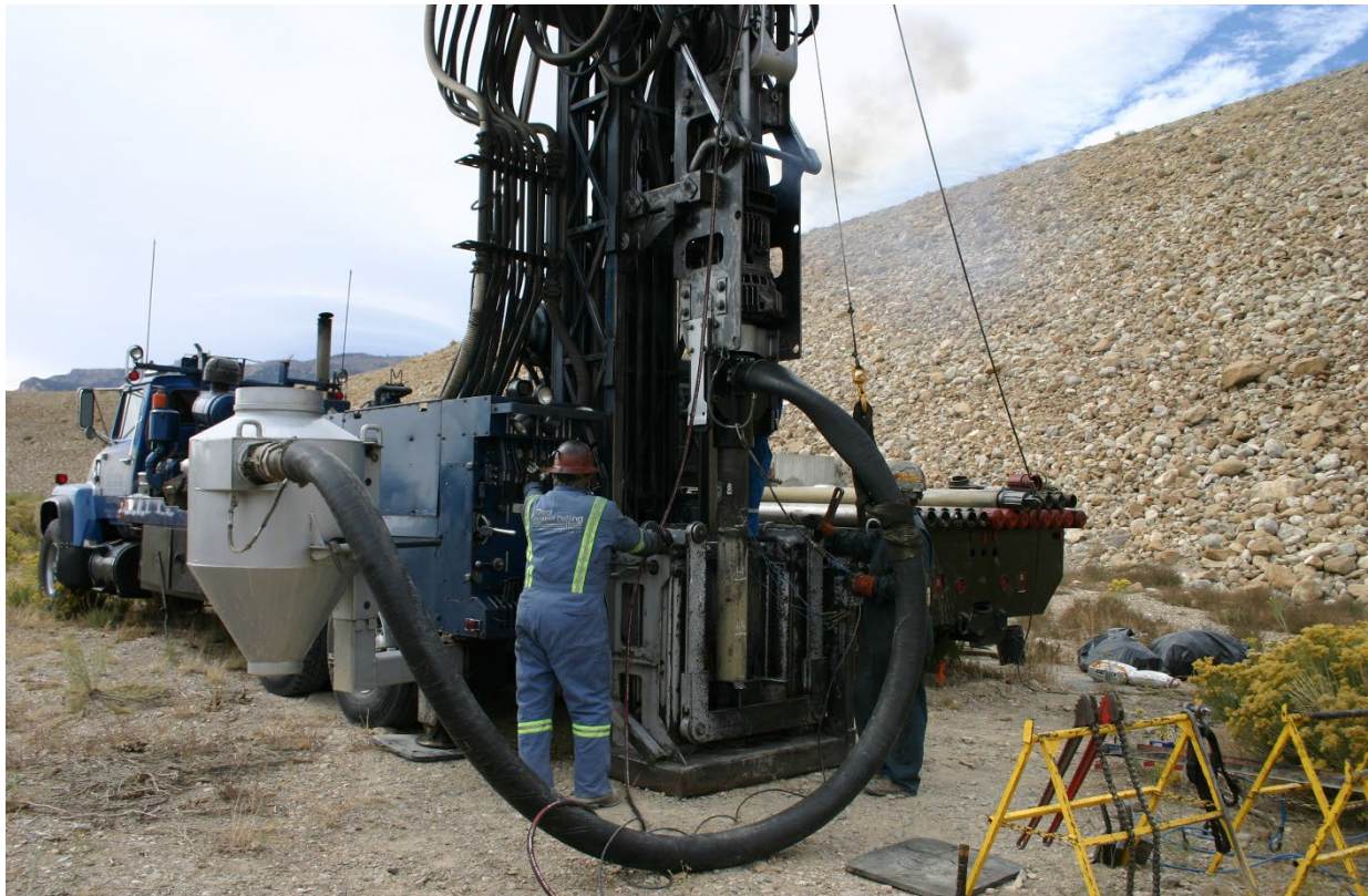
Figure 35. Energy measurements being acquired on the drill string during Becker Penetration Testing.
