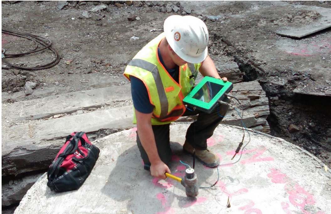
Figure 20. Typical low strain pile integrity test
