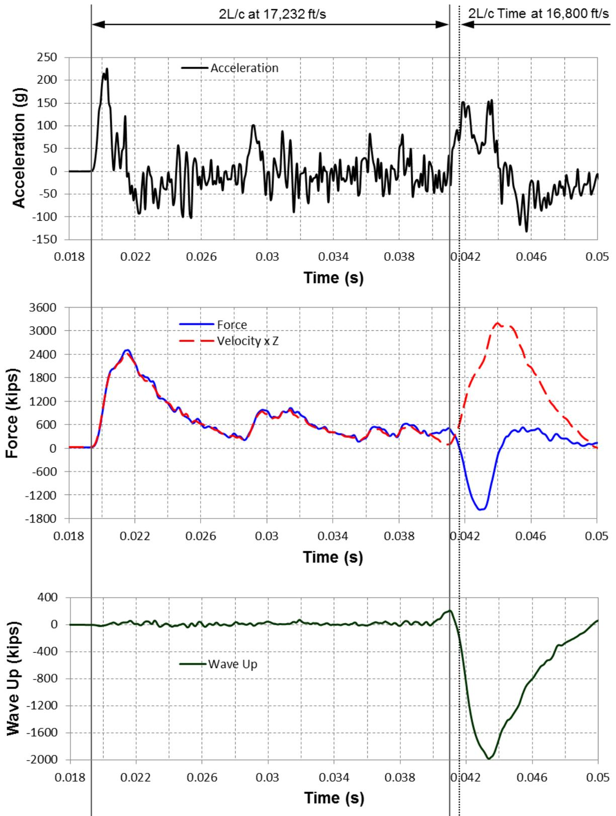
Figure 6. Case 4 – Acceleration (top), Force and Velocity Records (middle) and Wave Up (bottom) for Blow 3 in Early Easy Driving Conditions. Wave Speed of 17,232 ft/s (5,252 m/s).
