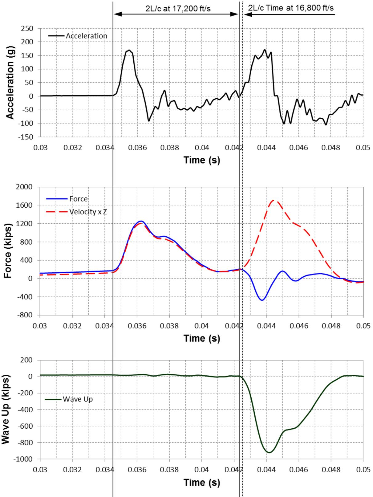
Figure 4. Case 2 – Acceleration (top), Force and Velocity Records (middle) and Wave Up (bottom) for Blow 6 in Early Easy Driving Conditions. Wave Speed of 17,200 ft/s (5,243 m/s).
