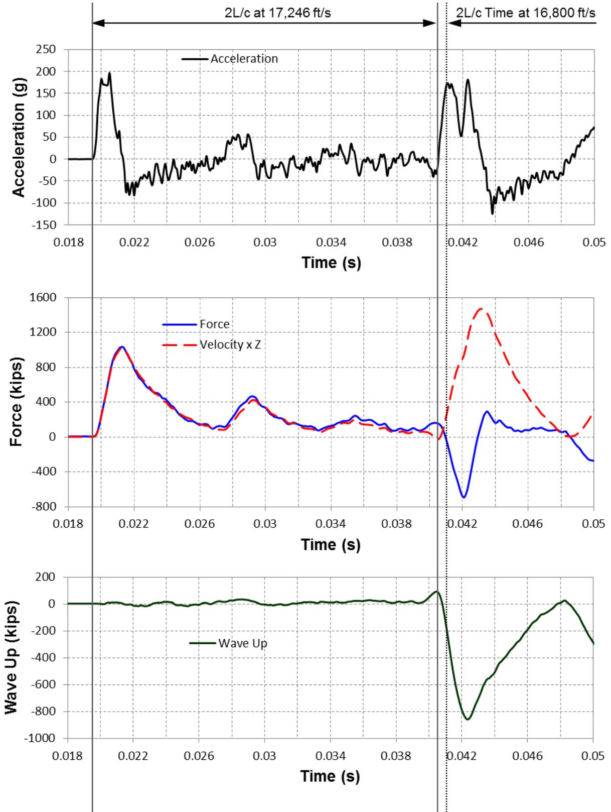
Figure 5. Case 3 – Acceleration (top), Force and Velocity Records (middle) and Wave Up (bottom) for Blow 2 in Early Easy Driving Conditions. Wave Speed of 17,246 ft/s (5,257 m/s).
