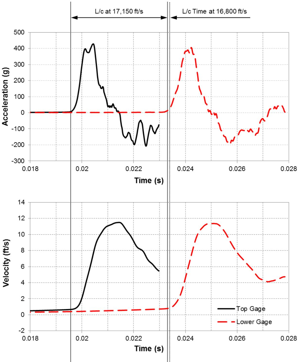
Figure 1. Case 1 – Partial Acceleration Records (top) and Velocity Records (bottom) from Two Gage Attachment Positions Located 64.2 ft (19.6 m) Apart.
