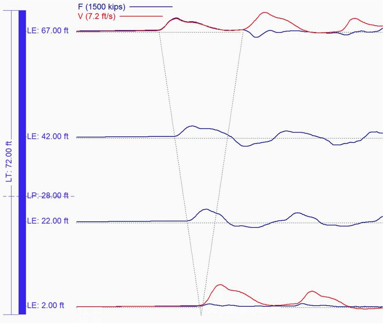
Figure 3. Case 2 - Wave Travel Past Multiple Gage Locations at Wave Speed of 17,200 ft/s (5,243 m/s).
