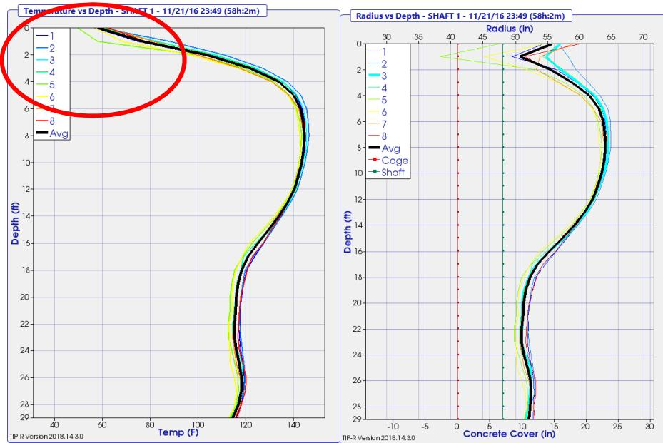
**Fig. 1 and 2 – Shaft 1 Temperature and Effective Radius versus Depth**
