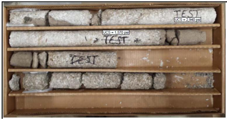
**Figure 6 - Shaft 2 Core Results**
