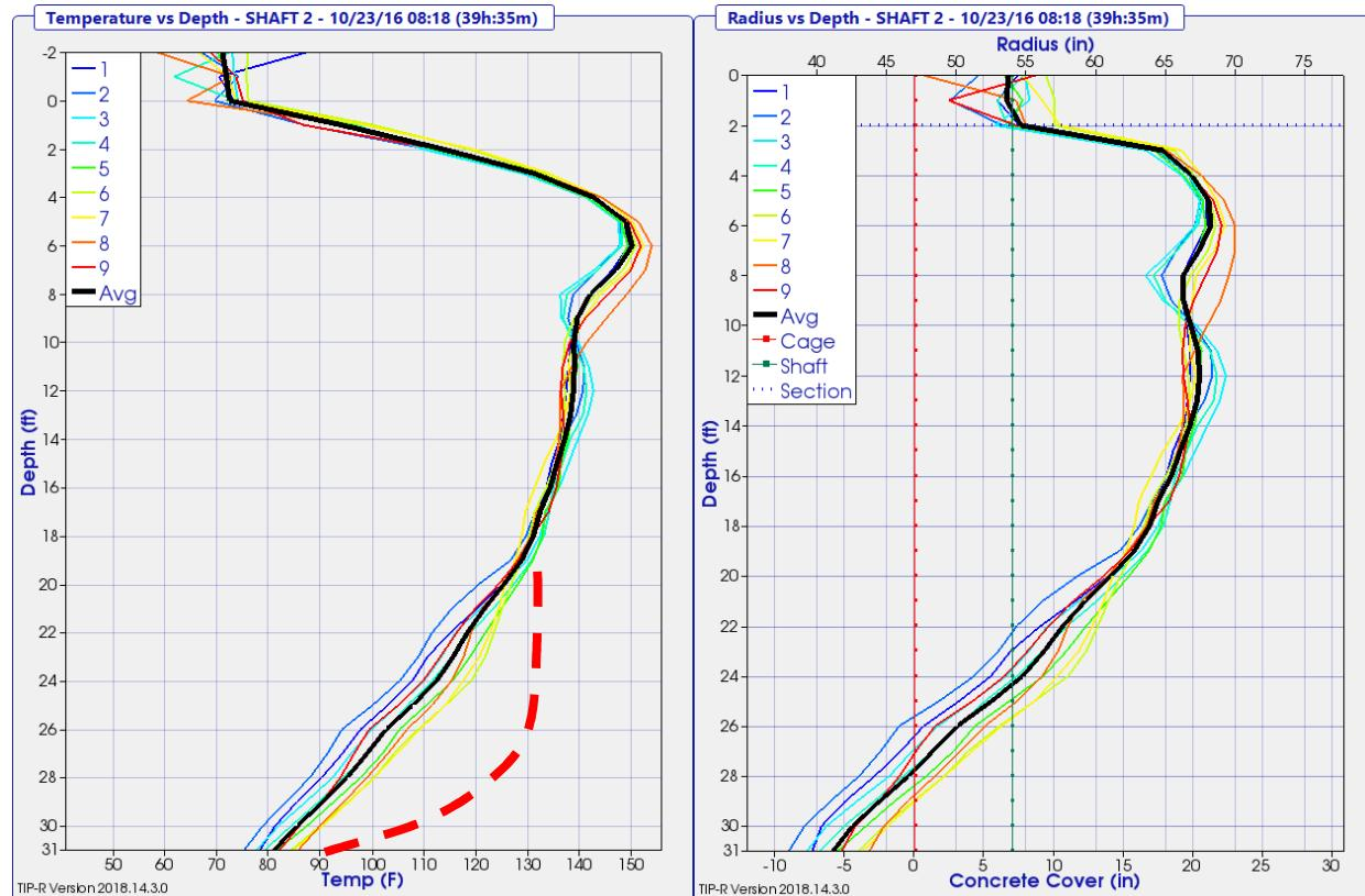
**Fig. 3 and 4 – Shaft 2 Temperature and Effective Radius versus Depth**
