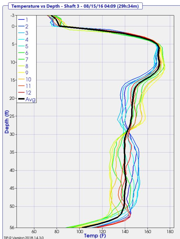
**Fig. 7 – Shaft 3 Temperature versus Depth**
