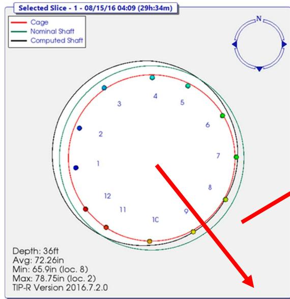
Figure 9 – Cross-Section of Shaft 1 at 36-ft Depth
