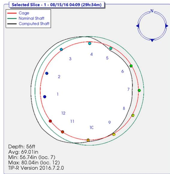
Figure 10 – Cross-Section of Shaft 1 at 56-ft Depth (Bottom of Pier)
