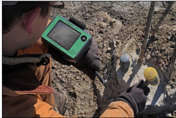
FIG 1. Pile Integrity Tester with Instruments
