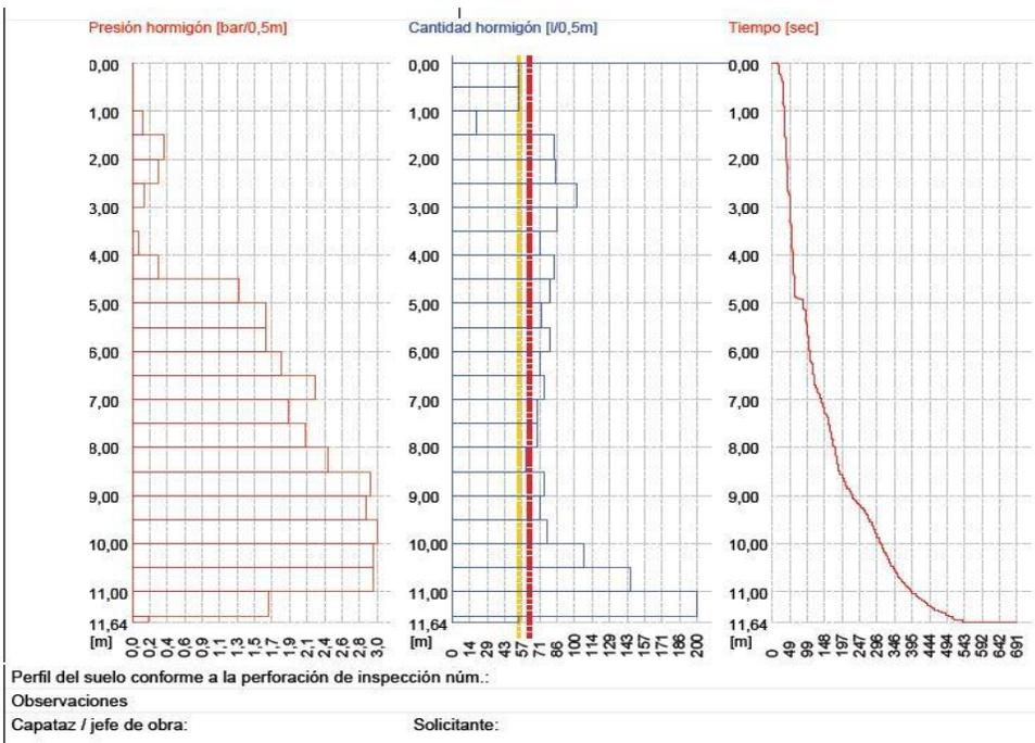
Figure 20: TP2- Bolivia, Concrete pressure (left), concrete volume (middle), concreting time (right)
