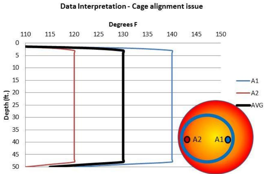
**Figure 7: Temperature shift between wires A1 and A2 due to cage misalignment.**
