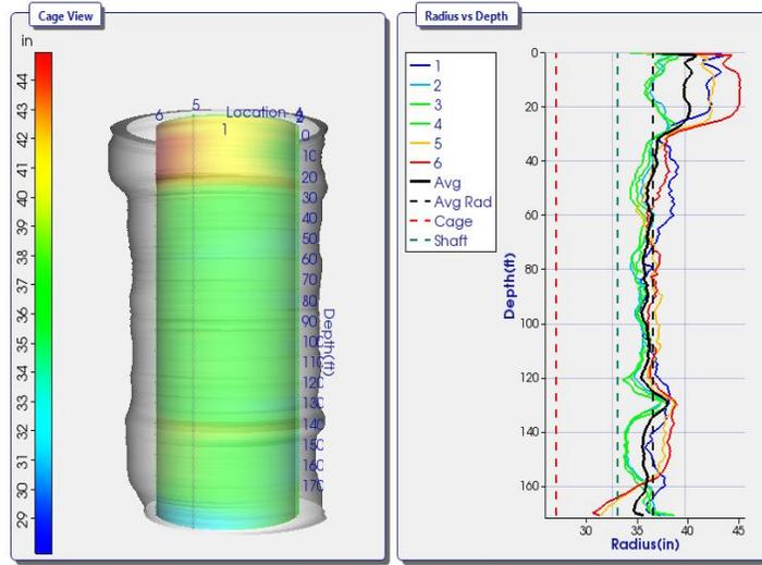
Figure 16: Innerbelt Test Shaft – Shaft shape as derived by TIP including location of the reinforcement cage (left), radius vs. depth profiles as calculated by TIP (right).
