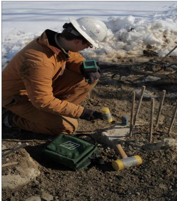
**Figure 4: Low strain integrity test equipment and configuration (PIT-X Unit)**
