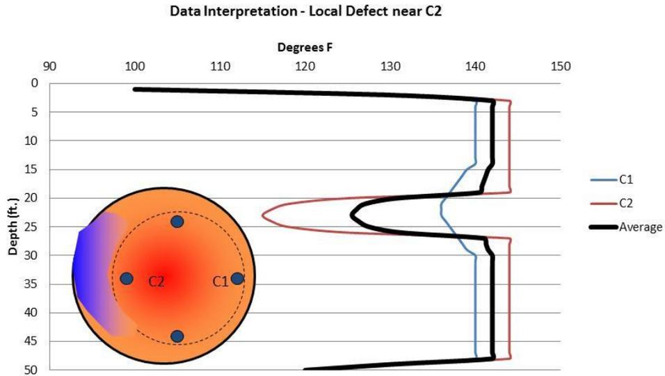
**Figure 6: Temperature drop at around 20 ft due to the presence of defect.**
