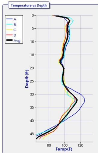
**Figure 11: Shafts A – Measured Temperatures (4 wires and average).**
