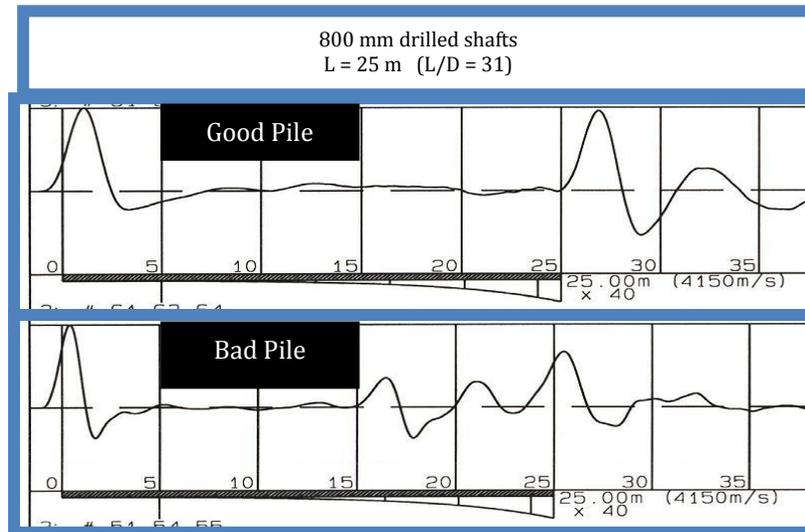
Figure 5: Low Strain Integrity Results depicting a good (top) and a bad (bottom) pile respectively.
