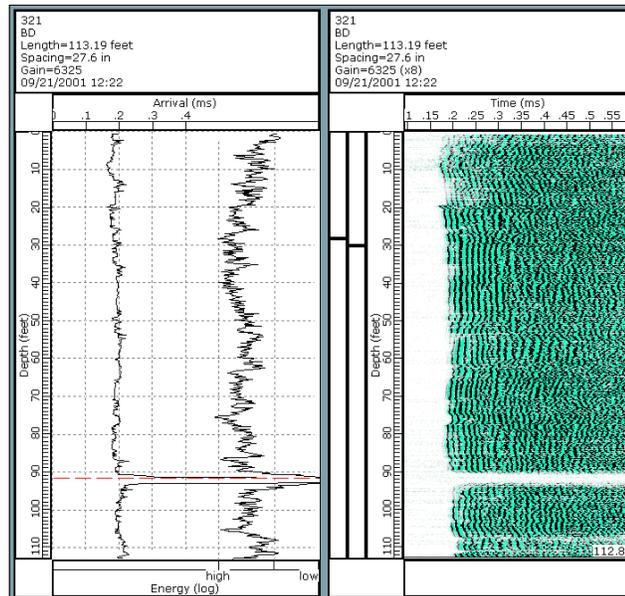
**Figure 2: CSL output depicting a defect at around 90 ft below pile top.**
