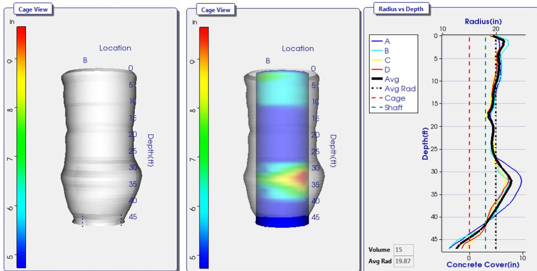
**Figure 12: Shafts A – Radius vs. depth estimation and 3-D Imaging.**
