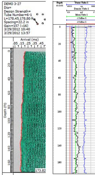
Figure 17: Innerbelt Test Shaft – CSL and GGL Sample Results.
