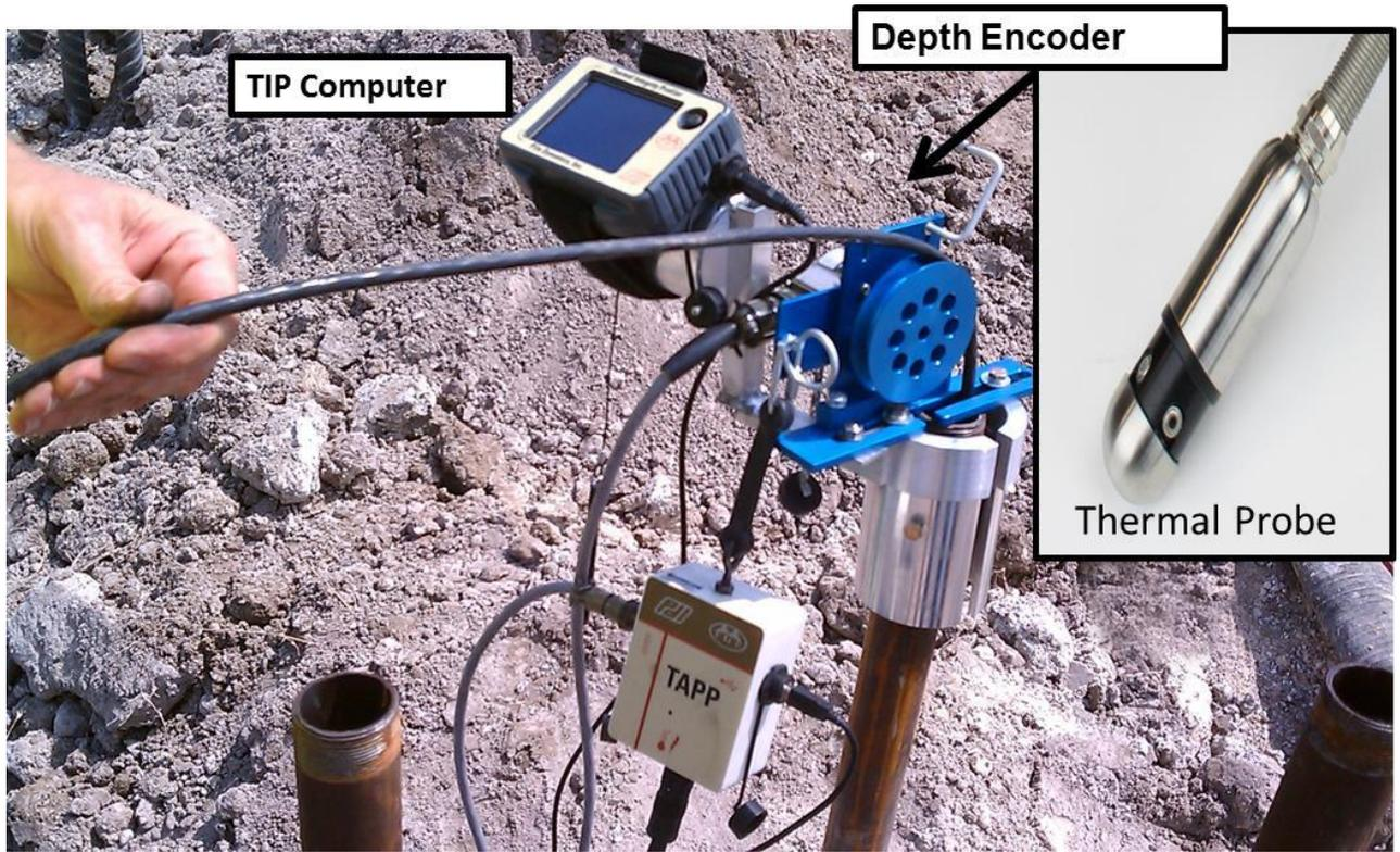
Figure 8: Thermal Integrity Profiler test configuration (probe method)
