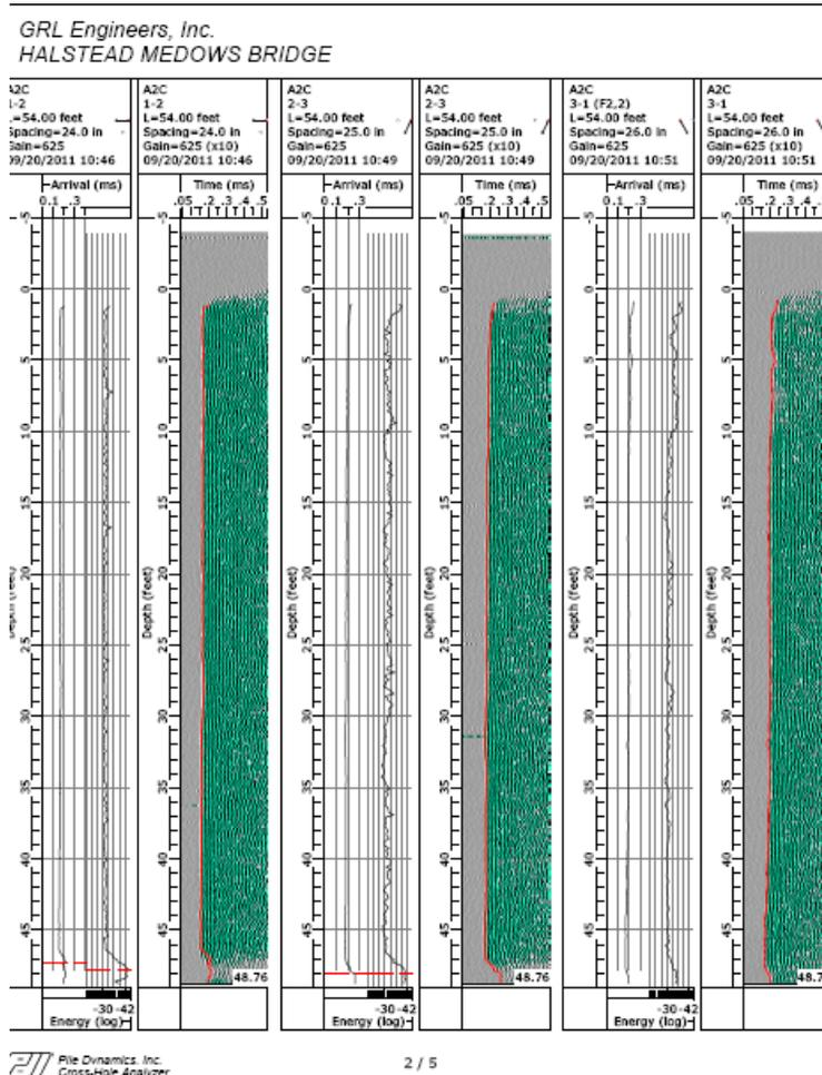
**Figure 13: Shafts A – CSL Test Results.**
