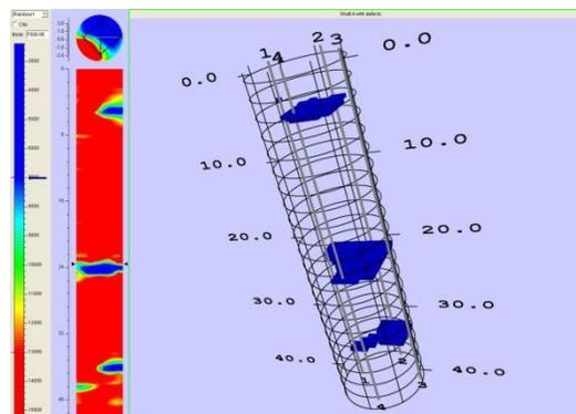
**Figure 3: Tomography display of CSL records showing defects**
