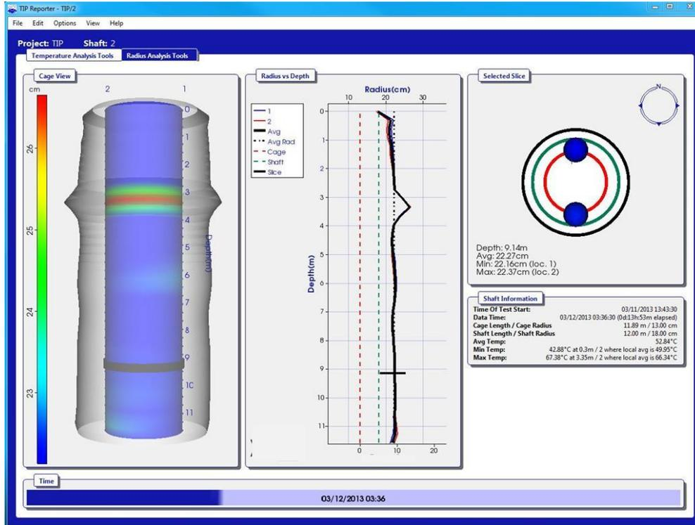
Figure 19: TP2, Bolivia – Radius vs. depth estimation and 3-D Imaging.
