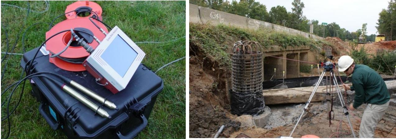
**Figure 1: CSL Testing equipment (left), a GRL engineer performing CSL testing (right)**
