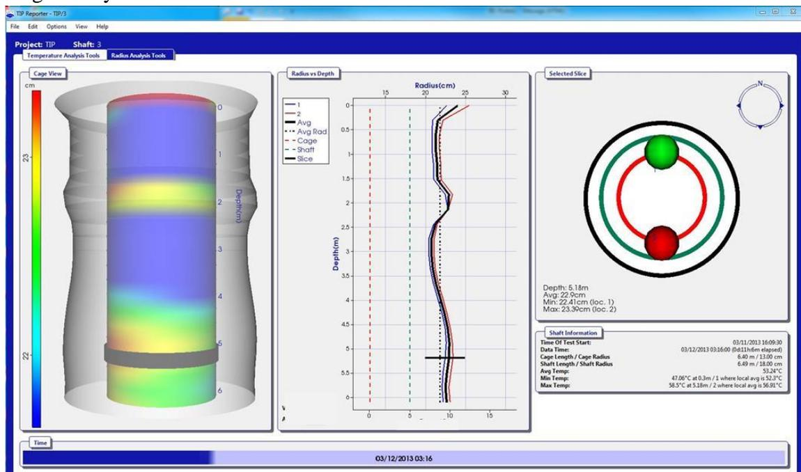
**Figure 21: TP3, Bolivia – Radius vs. depth estimation and 3-D Imaging.**
