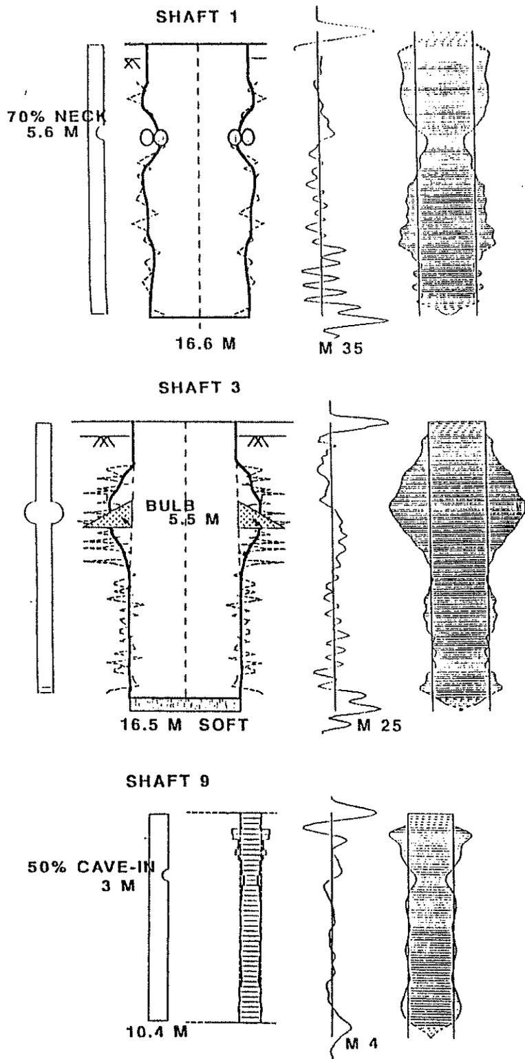
Figure 1. As planned (left), as built (Shafts 1 and 3), PITWAP signal match (Shaft 9), P.I.T. velocity signals (with magnification M), and shaft impedance profiles (right).
