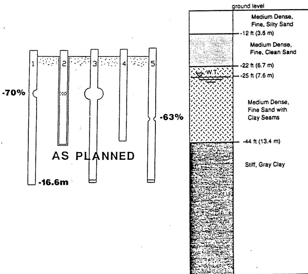
Figure 2. Impedance Profiles versus shaft "As Planned"
