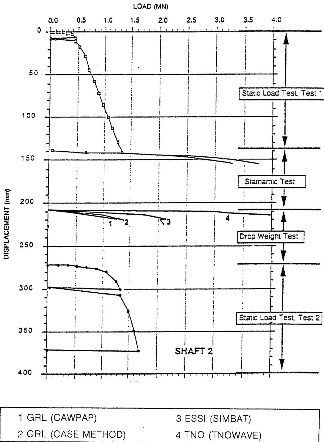
Figure 4. Shaft 2, Load versus Displacement (after Baker 1993)
