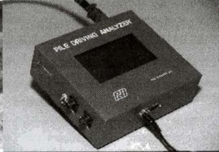
Abb 3: Pile Driving Analyzer, Model PAL
