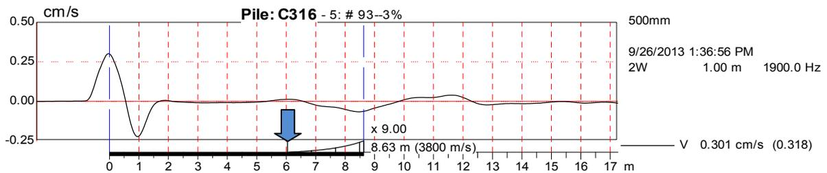
**Figure 8 Inappropriate MD – Defective Pile appears OK**
