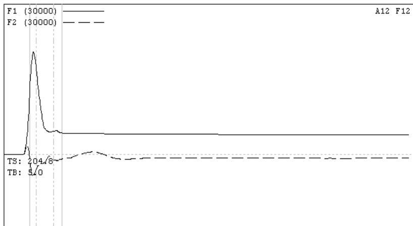
Figure 4 - Bad F1 strain data force is well positive at end – Cracked Pile Top
