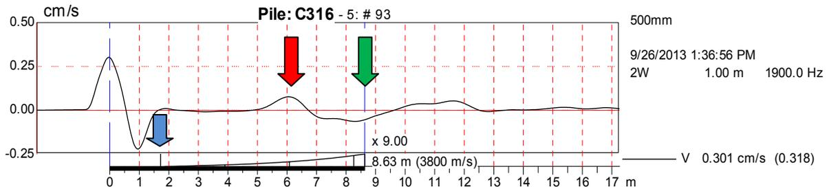
**Figure 7 Appropriate MD – Defective Pile**
