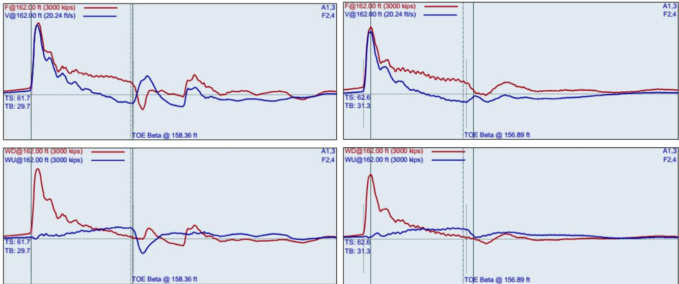
**Figure 1.** Force and velocity / Wave-up and Wave-down data from 7-day restrike testing
