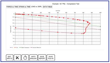
Load vs Displacement report on a recent Static Load Test
