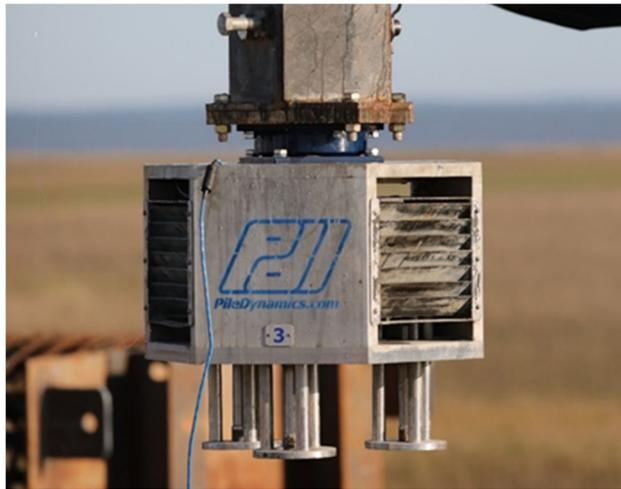
Fig 7. Shaft Quantitative Inspection Device.
