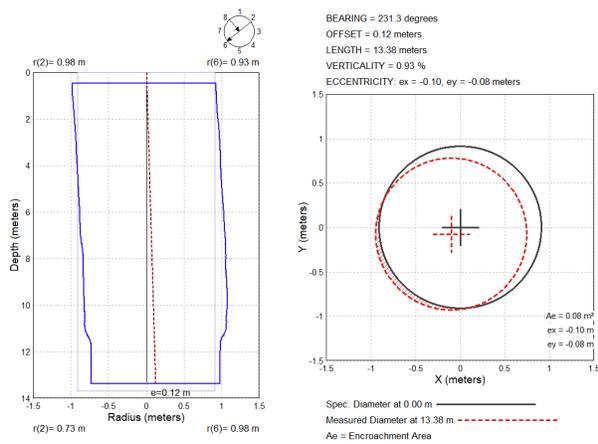
Fig 5. Maximum calculated eccentricity and resulting excavation verticality.
