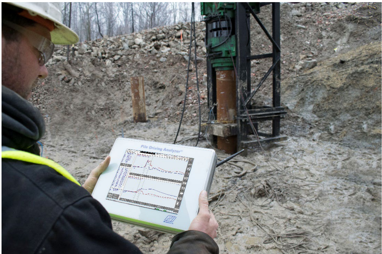
Figure 2. Dynamic Pile Monitoring with PDA 8G and wireless data transmission during pile installation.
