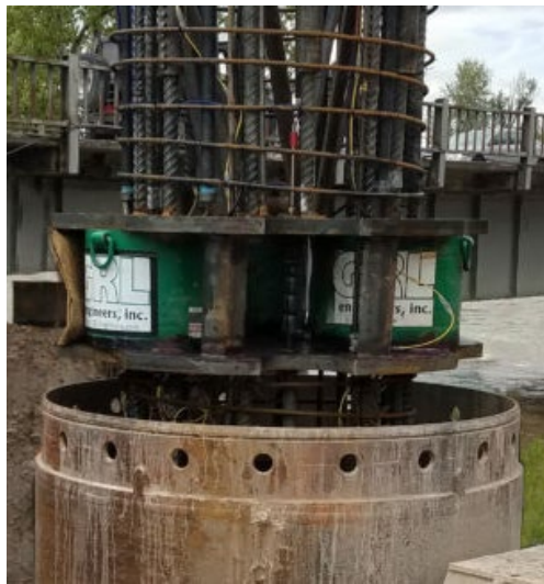
Figure 26. Installation in drilled shaft.
