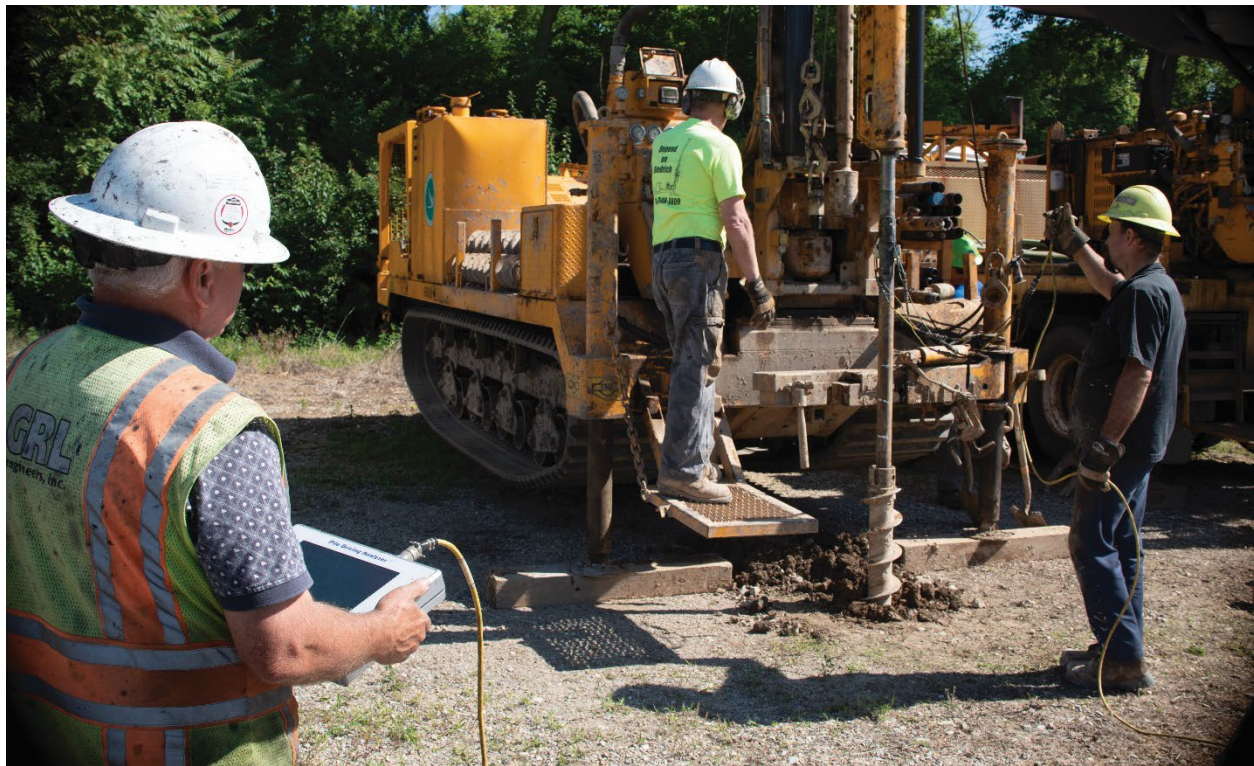
Figure 34. Energy measurements being acquired on the drill string during SPT soil sampling.
