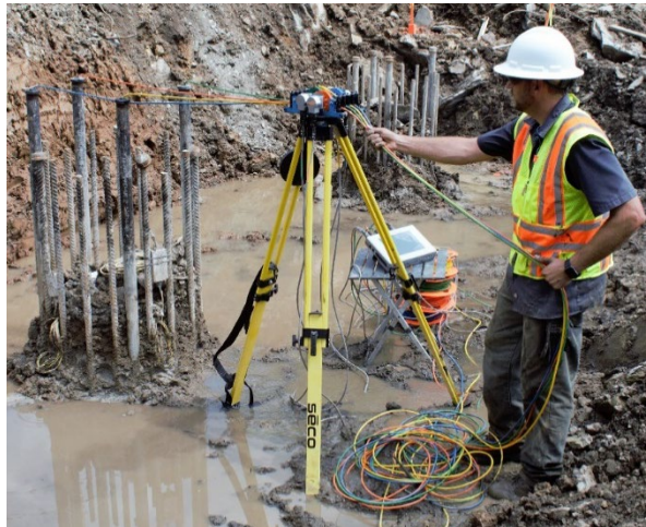
Figure 15. Typical field set-up of CSL test.
