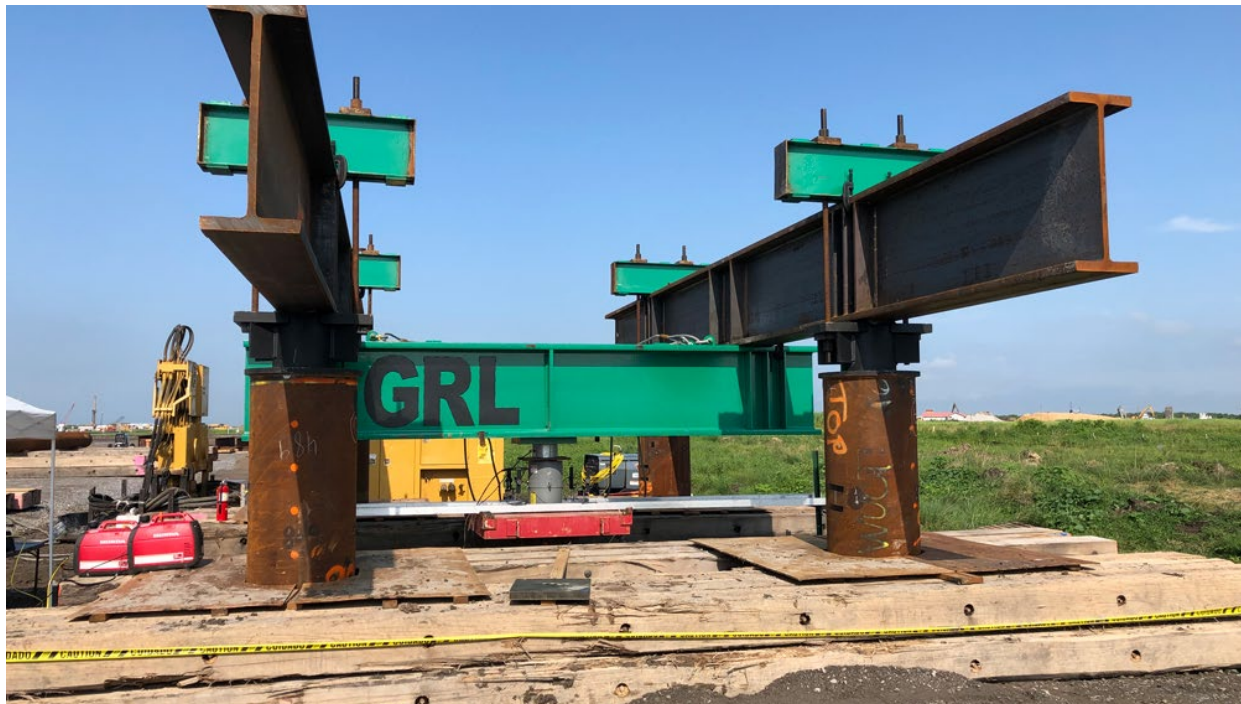
Figure 22. Reaction pile load frame for an axial compression load test.
