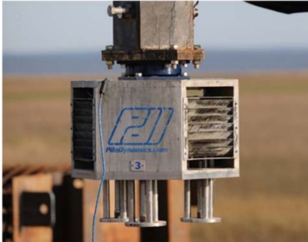
Figure 5. Shaft Quantitative Inspection Device
