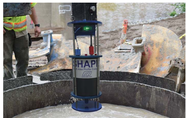
Figure 1. Shaft Area Profile Evaluator being lowered into a drilled shaft excavation
