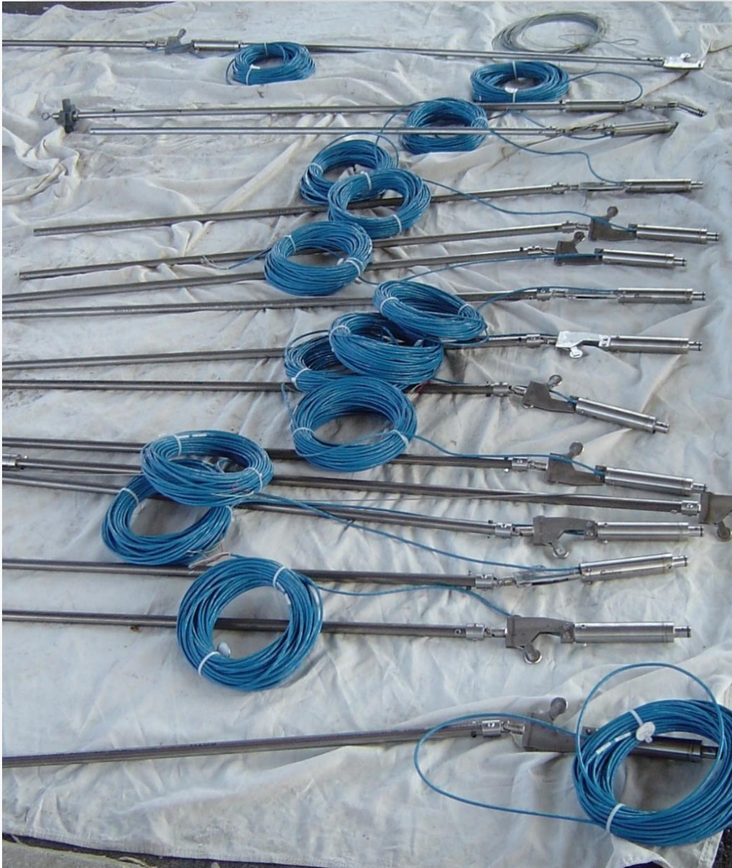
Figure 1. In-Place Inclinometer String Components Consisting of Connecting Rods, Wheel Assemblies, and Inclinometers.
