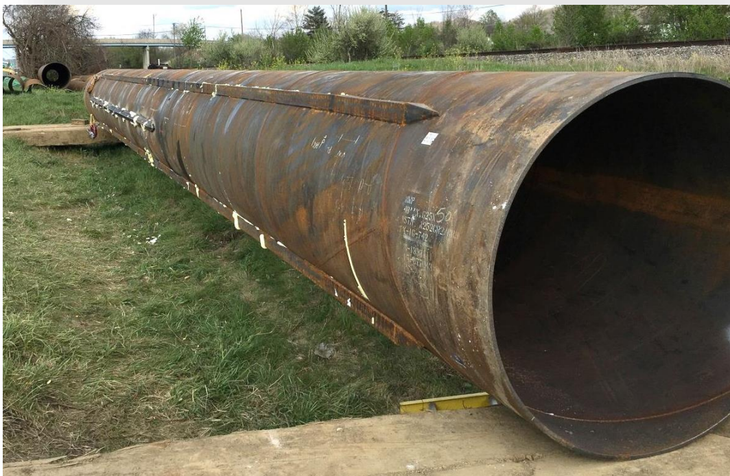
Figure 6. Completely Instrumented Open End Pipe Pile Ready for Driving.
