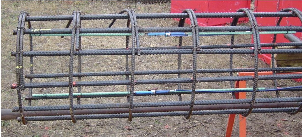
Figure 1. Vibrating Wire Strain Gage Sister Bars Attached to Reinforcing Cage.
