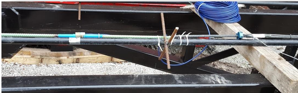
Figure 2. Sister Bar Mounted Strain Gages on Centering Rod. Vibrating Wire Strain Gage (on left) and Resistance Strain Gage and Accelerometer (on right).
