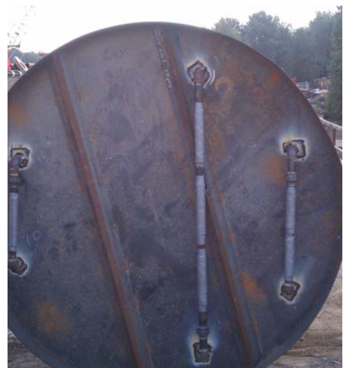
Fig. 2. Malcolm Drilling's tube-a-manchette system
