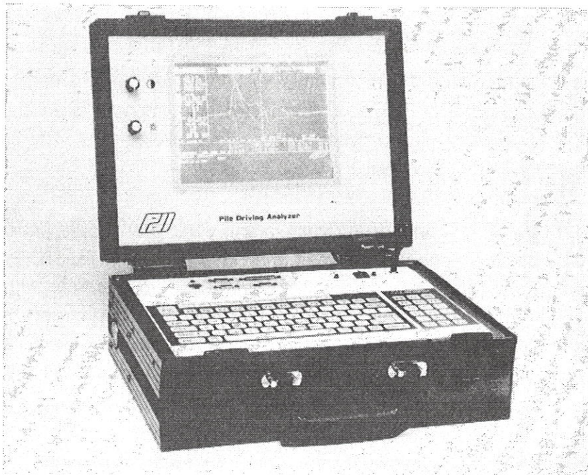
Figure 2: The Pile Driving Analyzer® (PDA)
