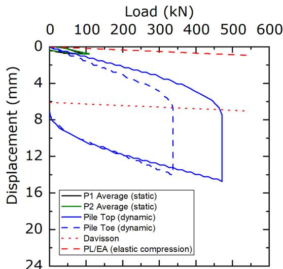
Figure 8. Results of Axial Load Tests on Fin Piles
