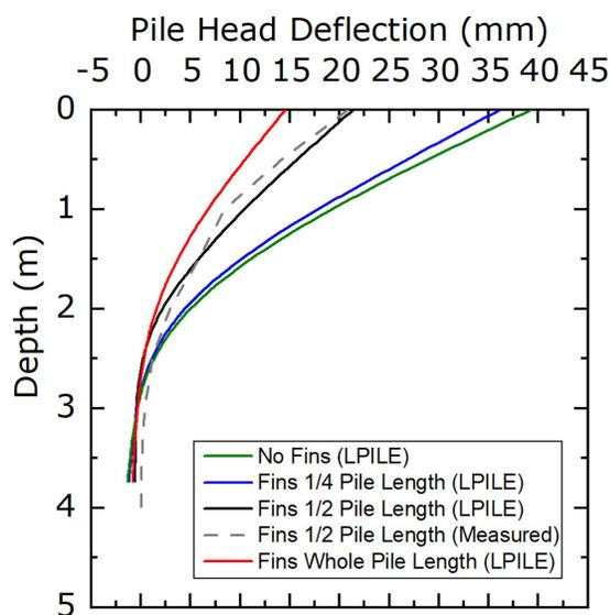
Figure 13. Parametric Evaluation of Changing Fin Length in LPILE
