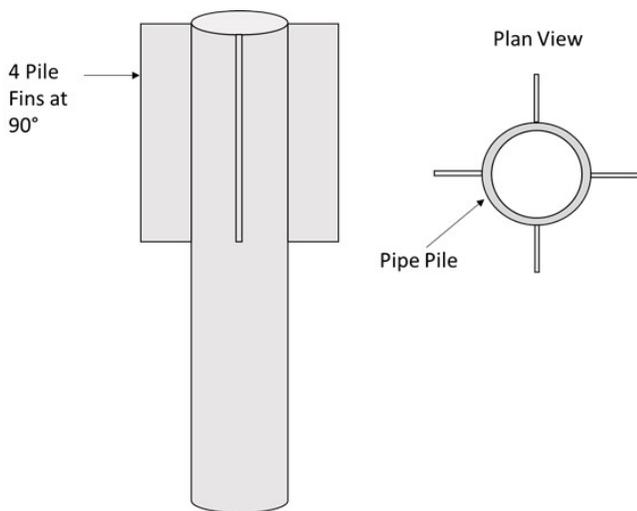
Figure 1. Example of Steel Fin Pile used in this Study
