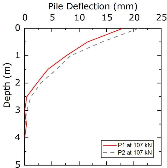
Figure 11. Lateral Load Test Deflection Comparison of P1 and P2
