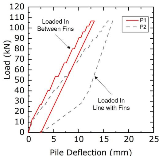
Figure 9. Lateral Pile Deflection Measured at the True Pile Head for P1 and P2
