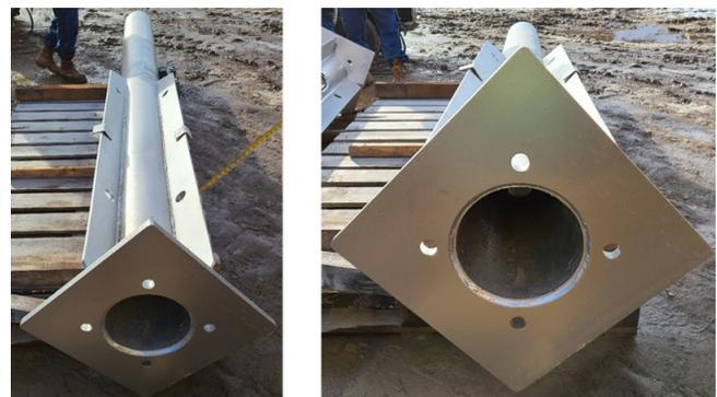
Figure 3. Photographs of Steel Fin Piles Tested in This Study
