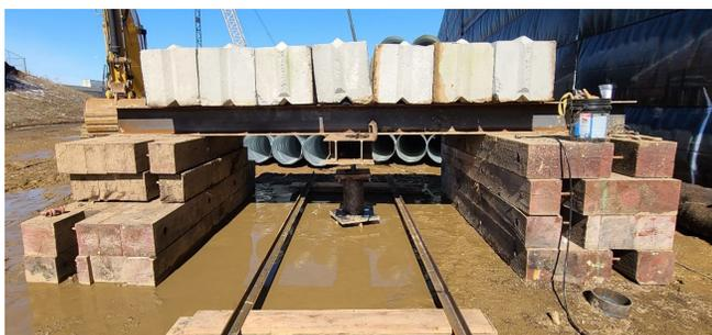
Figure 5. Photograph of Axial Load Test Setup
