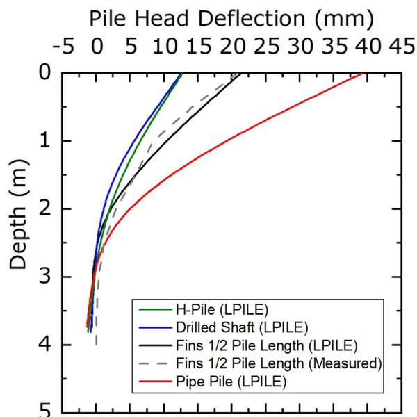
Figure 14. Parametric Evaluation of Pile Type in LPILE
