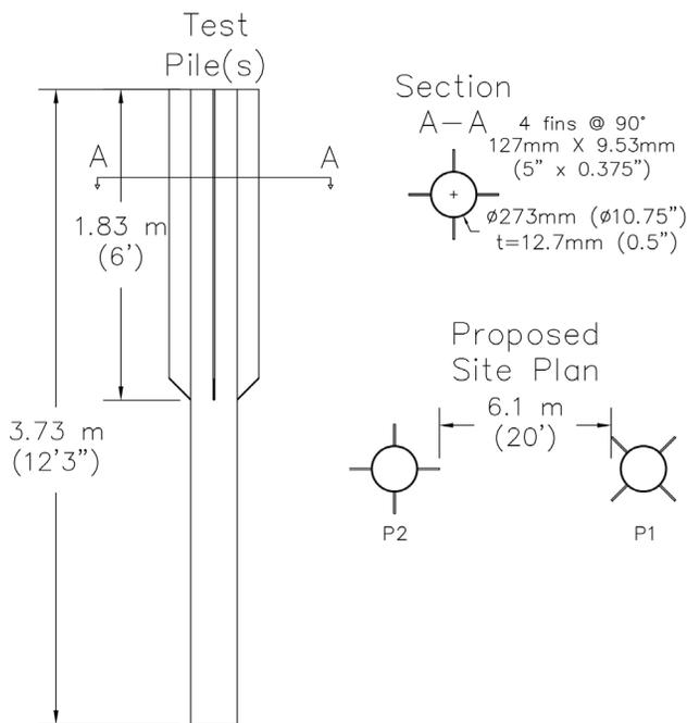
Figure 4. Schematic of Steel Fin Test Pile and Test Setup
