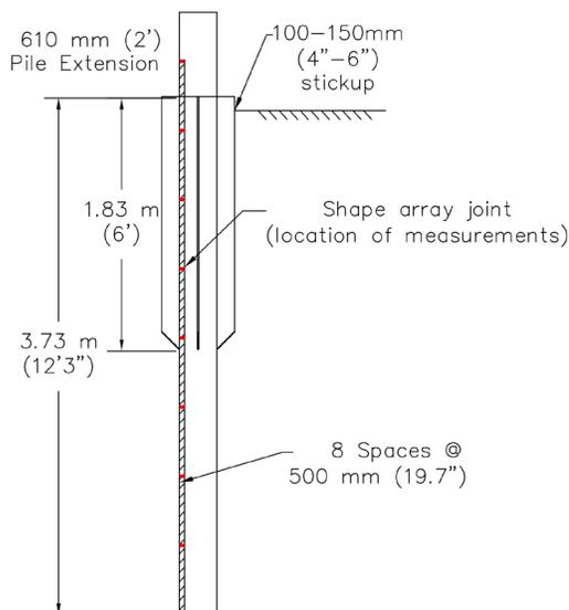
Figure 7. Schematic of Shape Array and Accelerometer Locations within Pile
