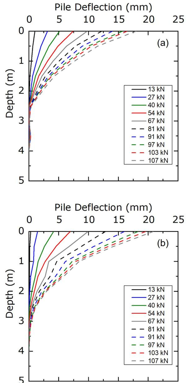
Figure 10. Lateral Load Test Results from Shape Array Measurements for (a) P1 and (b) P2
