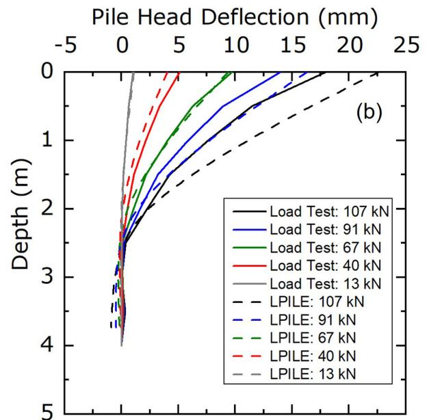
Figure 12. Lateral Load Test LPILE Model Comparison with Measured Deflections for (a) P2 loaded in line with fins and (b) P1 loaded in between fins
