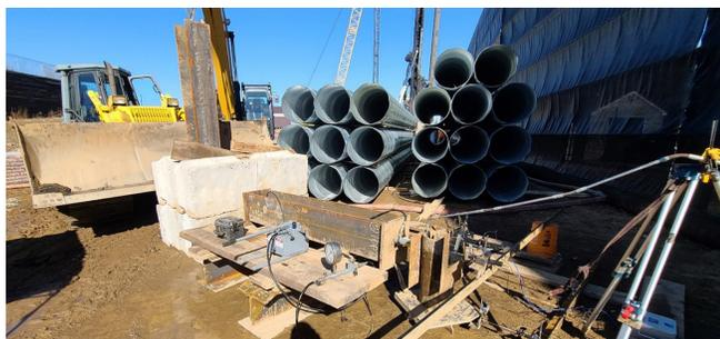
Figure 6. Photograph of Lateral Load Test Setup
