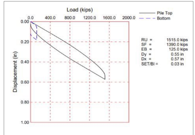
Figure 2. Load vs Displacement for prestressed concrete pile
