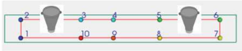
Fig.5 Configuration of thermal wires and tremie
