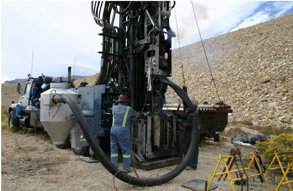
Figure 46. Energy measurements being acquired on the drill string during Becker Penetration Testing.
