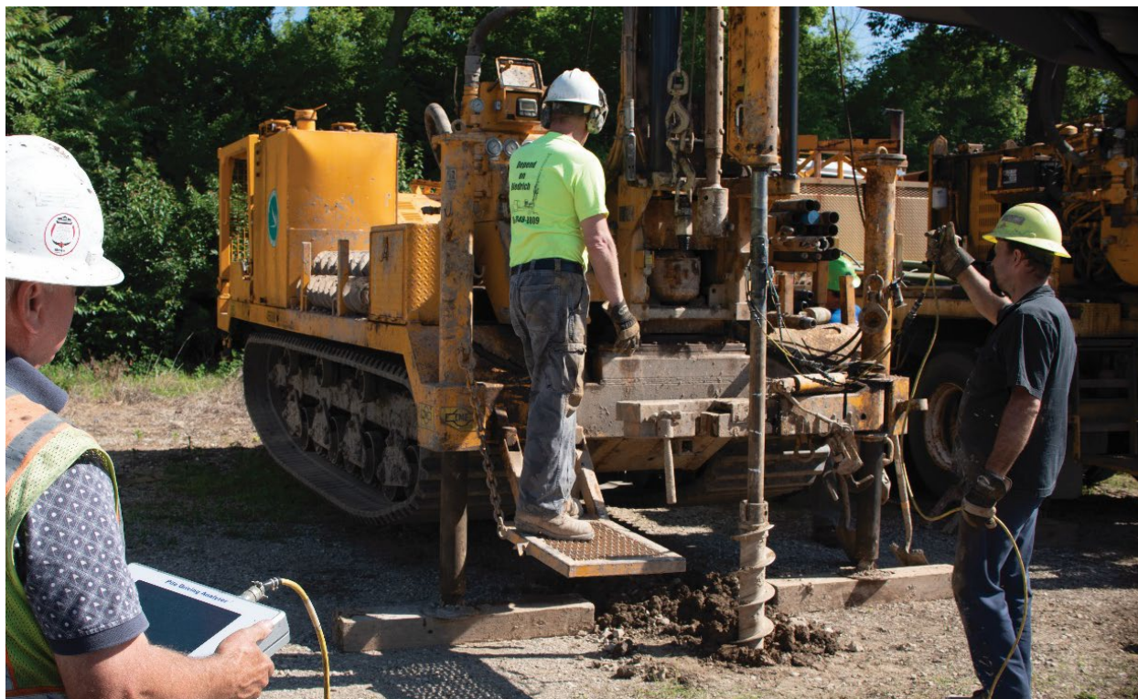
Figure 45. Energy measurements being acquired on the drill string during SPT soil sampling.
