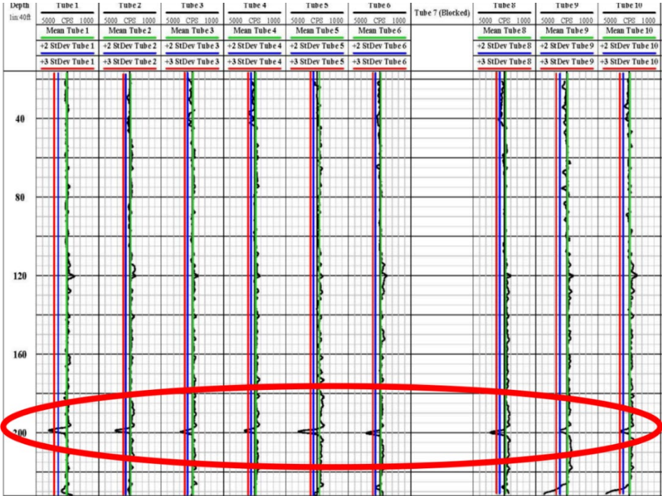
Figure 24. GGL results on a density vs depth plot.
